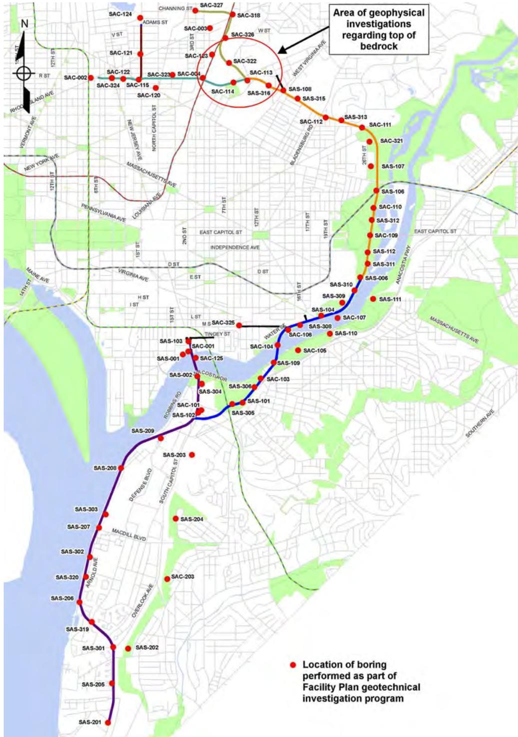
**Figure 9: Locations of Borings and Geophysical Survey**
