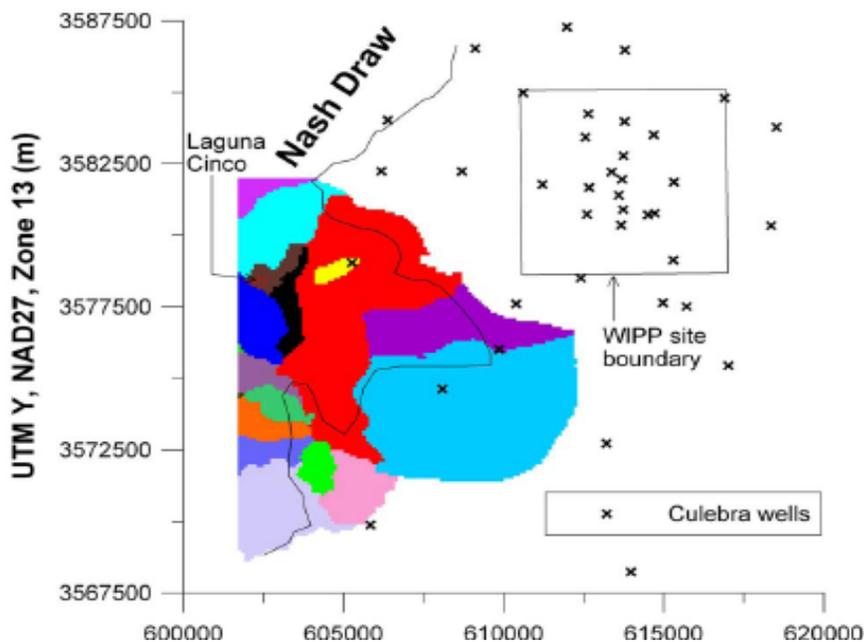
Figure 4- Catchment Basins, including Laguna Cinco, in Southeastern Nash Draw (CRA-2 Appendix HYDRO 2009, Fig. HYDRO-47).
