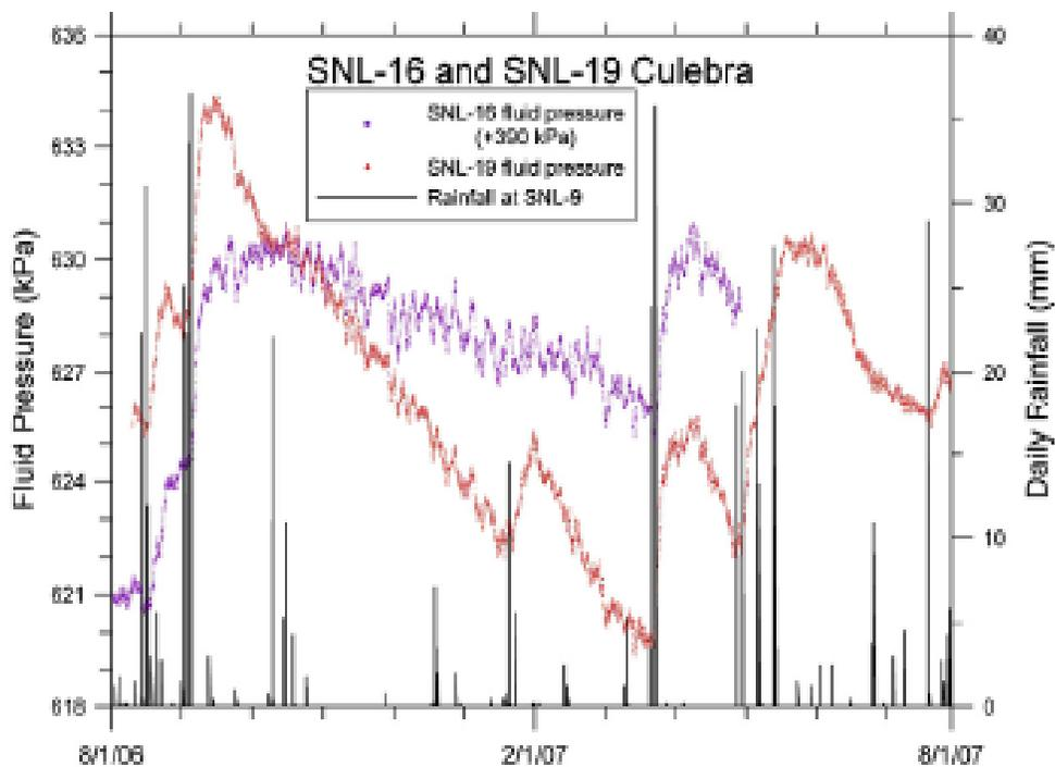
Figure 3. Rainfall Events Correlated with Nash Draw Shallow Groundwater Fluctuations (CRA-2009 Appendix HYDRO-2009, Fig. HYDRO-14).
