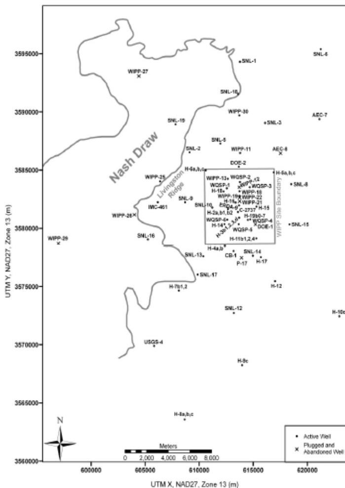
Figure 2 – Map of WIPP Site Boundary, Nash Draw, and Drill Hole Locations (CRA-2009 Appendix HYDRO-2009, Fig. HYDRO-1)
