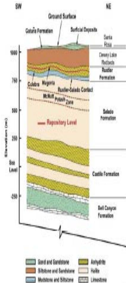
Figure 1. WIPP Geologic formations. (from CCA, 2006 – color added)
