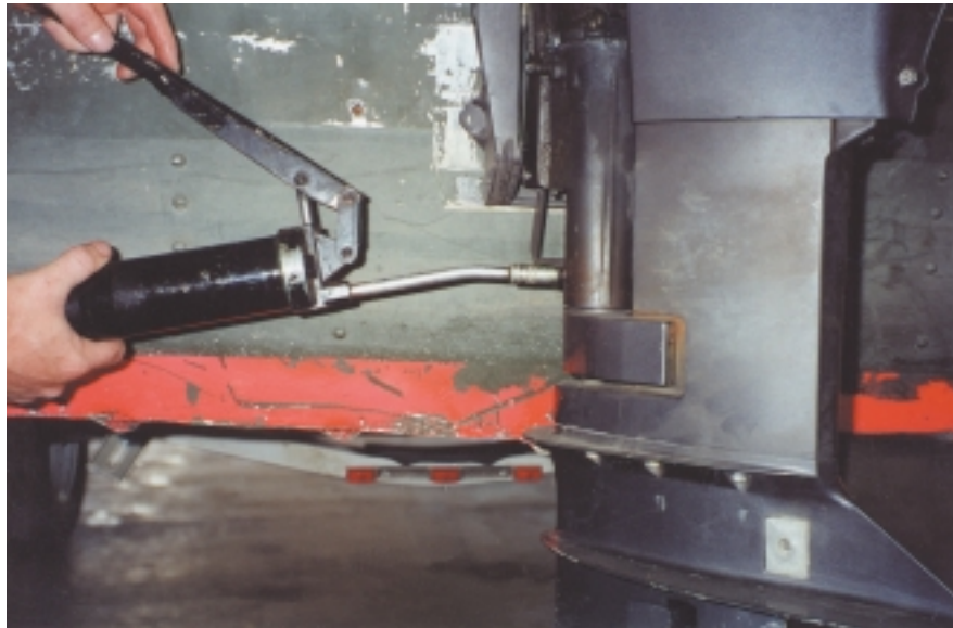
Figure 2-10. An outboard motor being lubricated.
