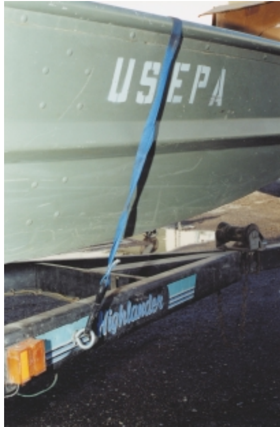
Figure 2-9. An eye bolt has been added to this trailer. This simple modification allows the boat to be securely fastened to the trailer with a ratchet strap so that the boat can be safely transported..
