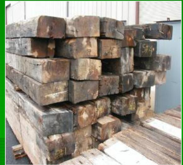
Reclaimed timber that can be milled into wood products
