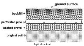
Effluent containing excessive amounts of grease, fats, and oils may clog the septic tank or drain field and lead to premature failure. The installation of *grease interceptors* is recommended for restaurants and other facilities with similar wastewater characteristics.
