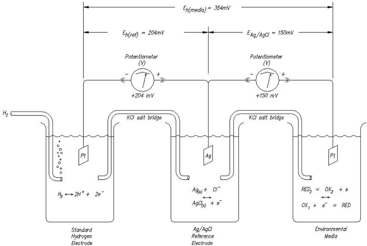
In Figure 5 below, a field instrument is represented as separate electrochemical cells. The Ag/AgCl reference electrode uses a ceramic frit or other means to provide the essential salt bridge to the environmental media. The platinum sensing electrode is immersed in the environmental media and connected internally in the instrument to measure the potential (voltage) between the two electrodes.
