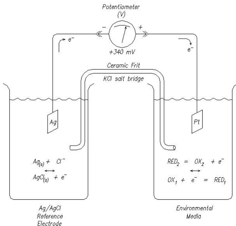
In this illustration, the ORP is measured as 340 mV. This measurement is made in reference to the Ag/AgCl reference electrode and would be reported as such, or as  $E_{Ag/AgCl} = 340\text{mV}$ .
