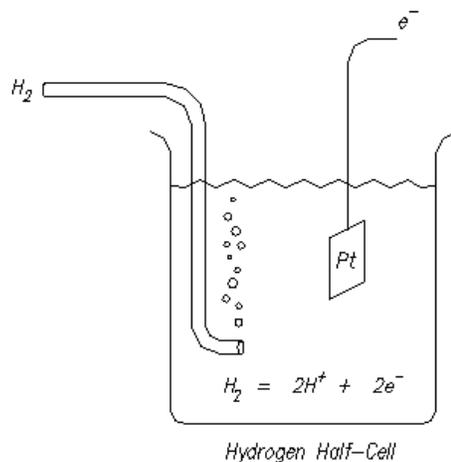
If, as shown in Figure 2, a SHE is connected with a salt bridge to a second half-cell in which a reduction reaction is taking place, the electric potential between the two cells can be measured. In the case shown, the potential of the right cell will be +0.34 Volts in reference to the standard hydrogen electrode on the left. This would be represented as an Oxidation Reduction Potential (ORP) of +340mV on the hydrogen scale, or simply as  $E_h = +340\text{mV}$ .
