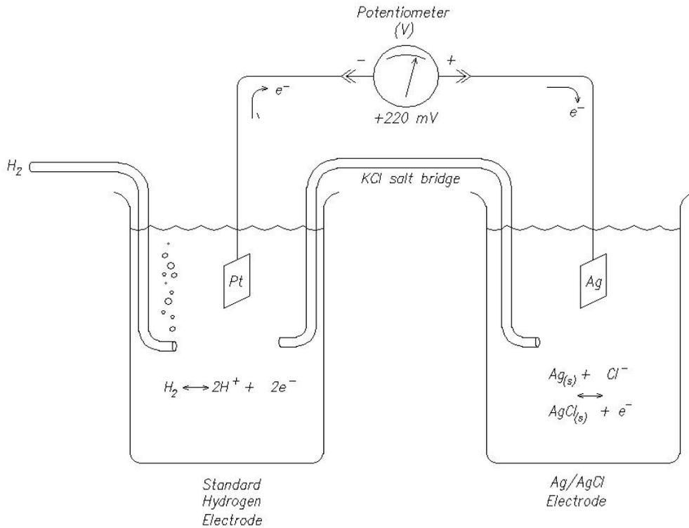
This half-cell potential of the Ag/AgCl electrode in reference to the SHE is used to convert measurements taken with an Ag/AgCl reference back to the hydrogen scale. While the laboratory Ag/AgCl half-cell shown has a potential of +220mV, practical reference cells have varying potentials based on temperature and filling solutions as shown in Table 1 below.
