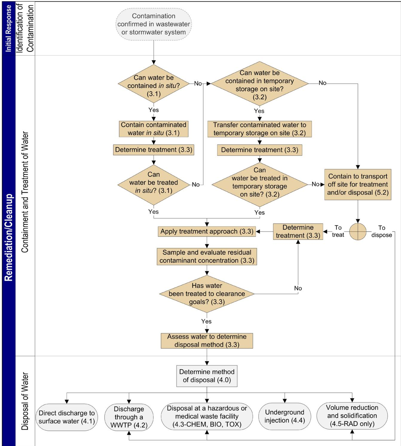
**Figure 3-2: Recommended Decision-Making Framework for Containment and Treatment of Contaminated Water for Wastewater and Stormwater Systems<sup>11</sup>**
