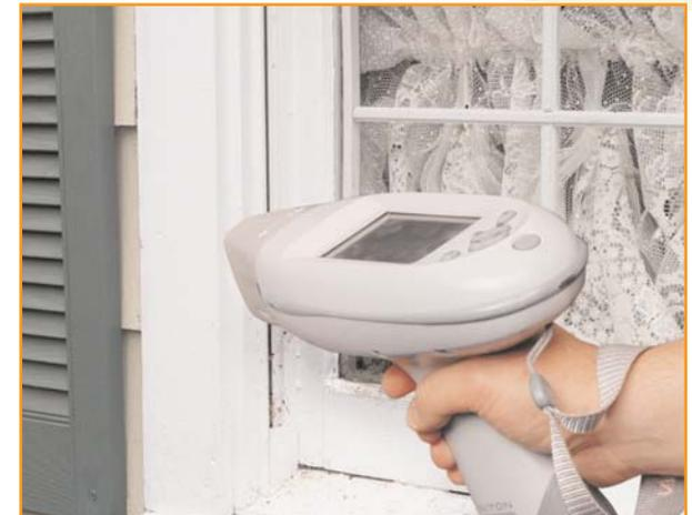
NITON's XLp 300 Series Lead Analyzer, pictured above, can measure the concentration of lead in paint even when covered by 50 or more layers of non-lead paint of unknown thickness and composition.
