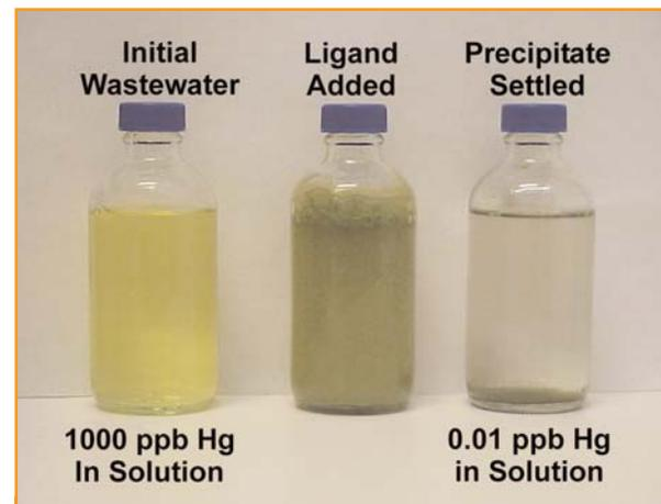
The FGS-MCX metal complex is insoluble in the aqueous phase, and thus precipitates efficiently in solution. The flocculation process is shown in the photograph above.
