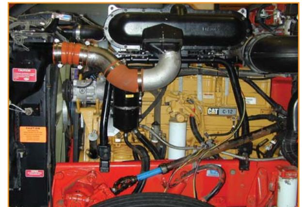
Membranes within the black housing mounted over the diesel engine pictured above generate NEA from cooled turbocharged air.
