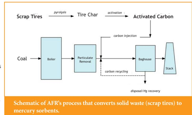
Schematic of AFR's process that converts solid waste (scrap tires) to mercury sorbents.
