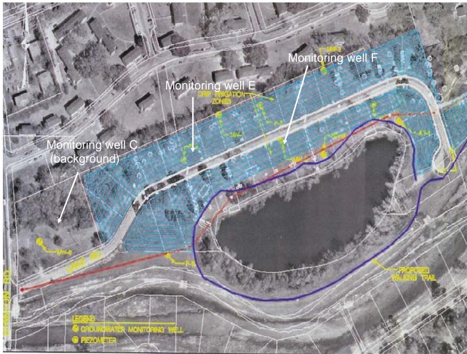
Figure 8. Ground water monitoring well locations.
