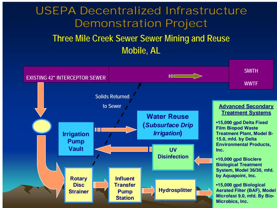
Figure 3. Schematic of the treatment process.
