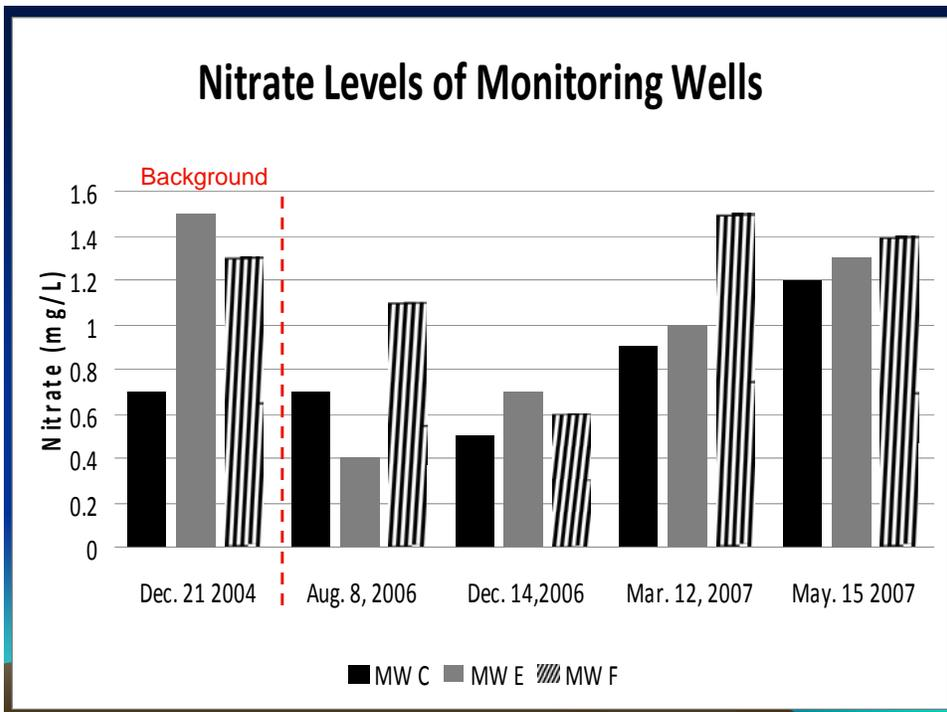
Figure 10. Nitrate concentrations in groundwater monitoring wells.
