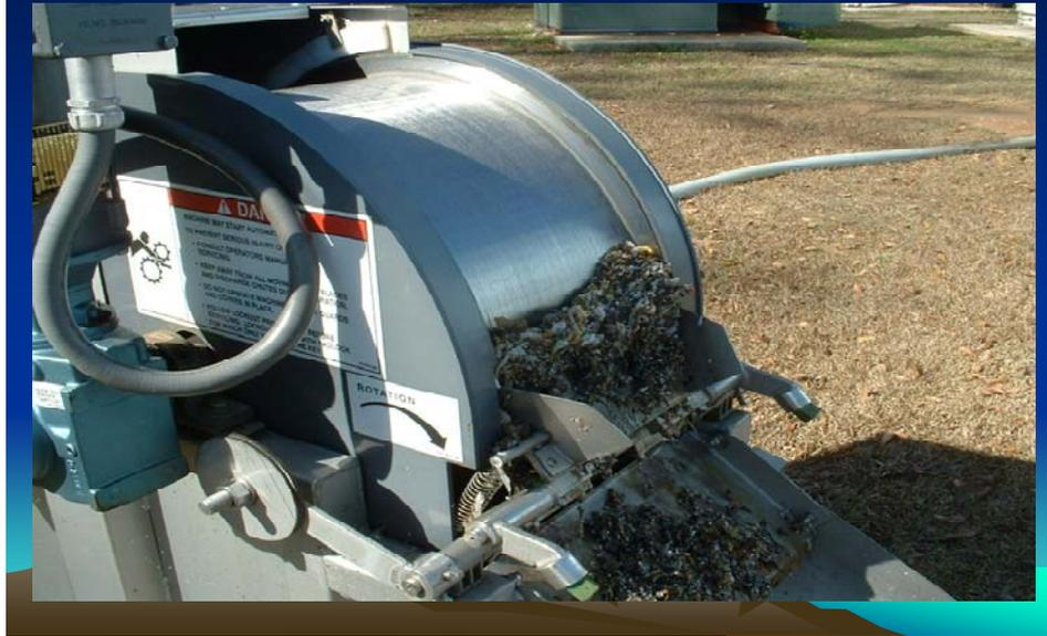
Figure 7. Hycor Rotostrainer rotary screen.
