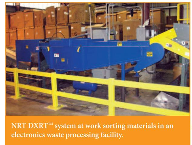
NRT DXRT™ system at work sorting materials in an electronics waste processing facility.
