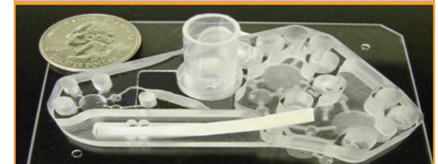
**Top:** Schematic of Card™ showing 6 pumps and 25 valves and general locations of the various functional components of the assay. **Bottom:** Photograph of fully integrated *CryptoDetect* CARD™.
