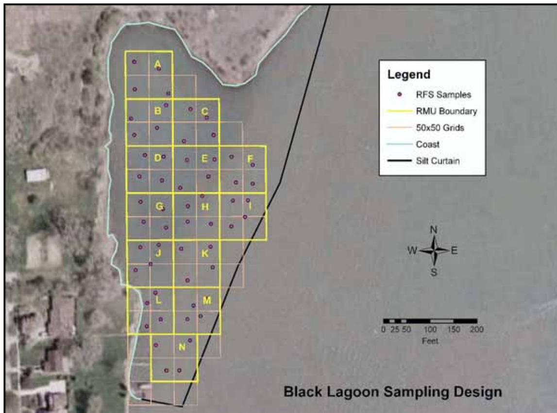
Figure 5-1 Black Lagoon Sediment Confirmation Sampling Design
