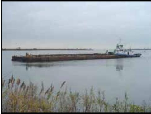
Three transport barges were used to convey the dredged materials to the government-provided CDF on Pointe Mouillee. The barges were moved using the *Robin Lynn*, a 90-foot, 1,800-horsepower tugboat, up the Trenton Channel to the north, under the Grosse Ile toll bridge, and into the Detroit River Channel.
