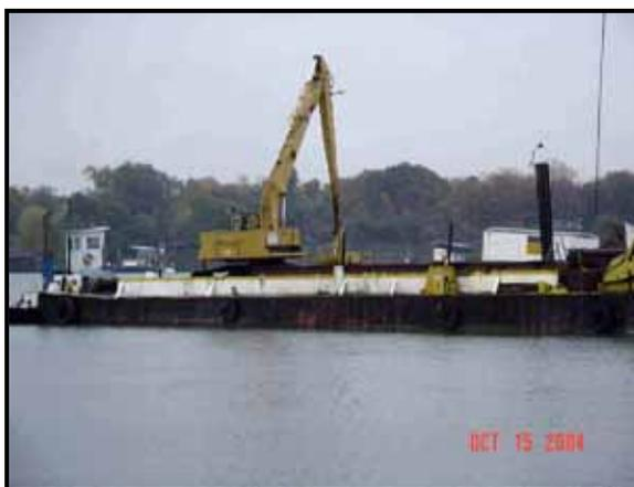
barge (dredge plant). The hoppers contained weep holes, which allowed necessary bulk dewatering of the sediment. Absorbent pads or sausage boom were placed on and around the hoppers to contain any oil. A silt fence and filter fabric panels were attached on the inside of the hoppers in front of the weep holes. This allowed the material to shed water, yet prevented as much re-suspension of the sediments as possible.
