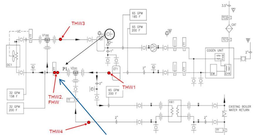
Placement of flow meter here would not capture UWHR
