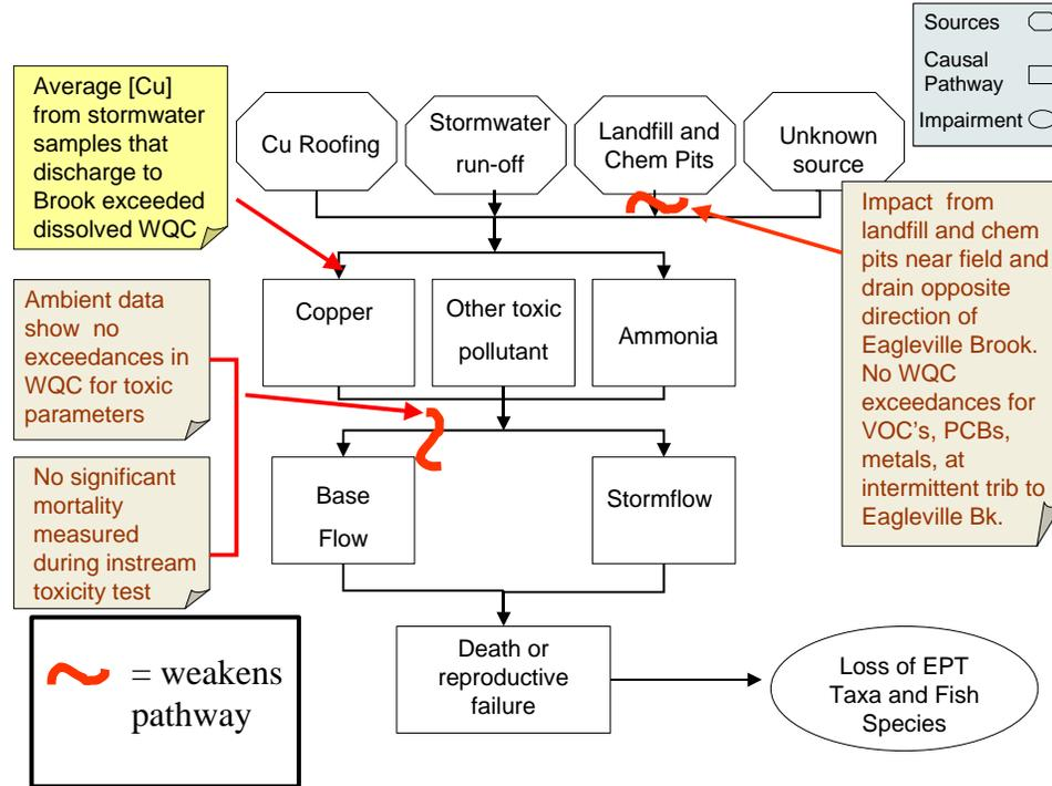
Figure 1. Conceptual model of toxic contamination as the cause of the low abundance of fish and EPT taxa. WQC is water quality criteria and refers to criteria as defined in Connecticut's Water Quality Standards<sup>9</sup>.
