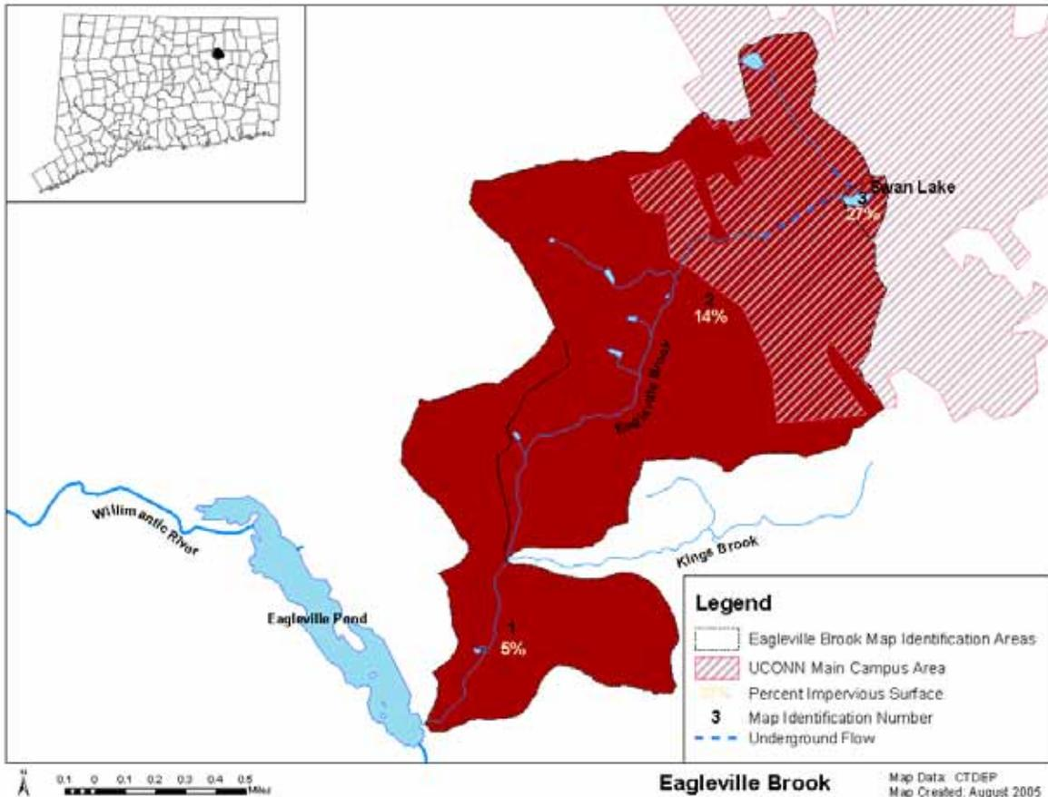
Figure 3. Eagleville Brook watershed showing the Map Identification Numbers 1-3 and the corresponding % IC values derived using ISAT from the 2002 Land Cover data.
