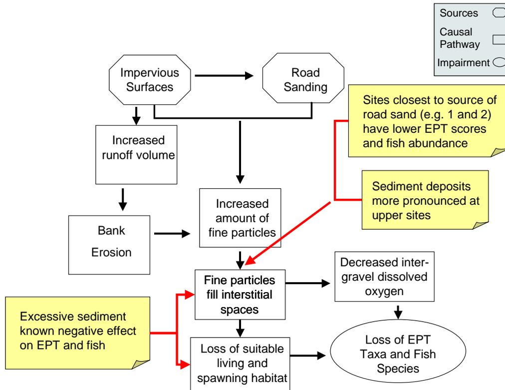
Figure 2. Conceptual model of embedded substrate as the cause of the low abundance of fish and EPT taxa.
