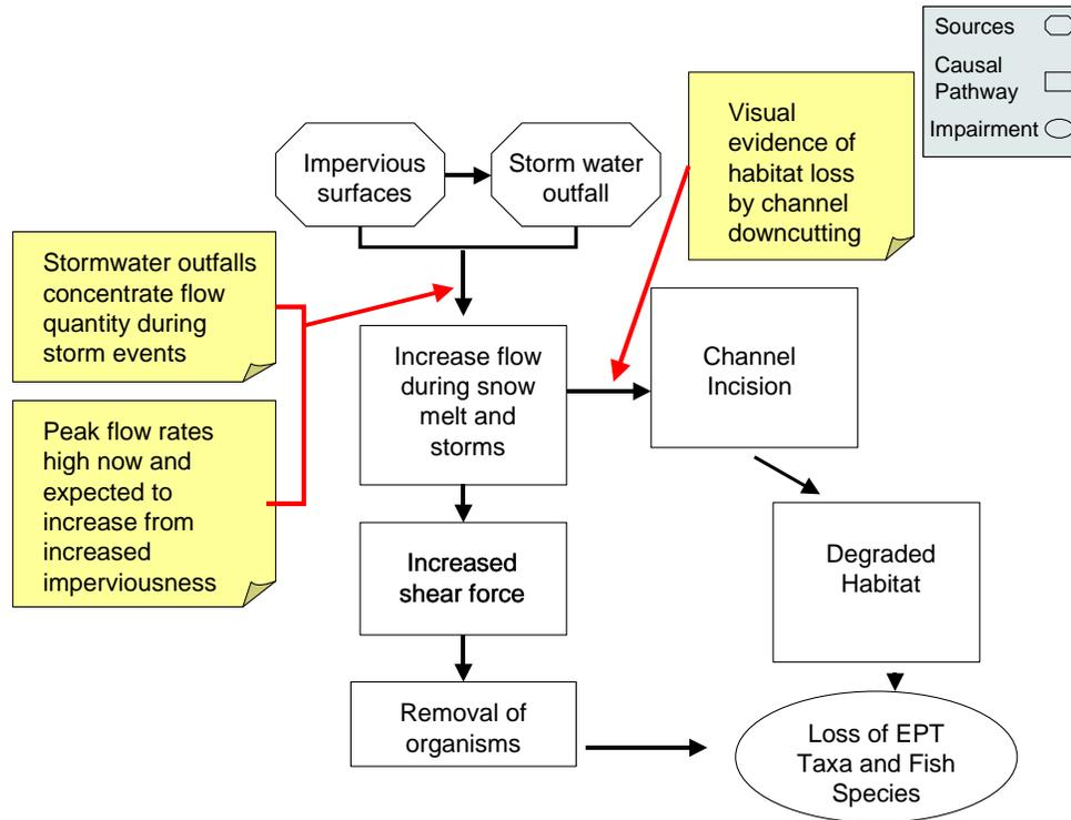
Figure 3. Conceptual model of high flow as the cause of the low abundance of fish and EPT taxa.
