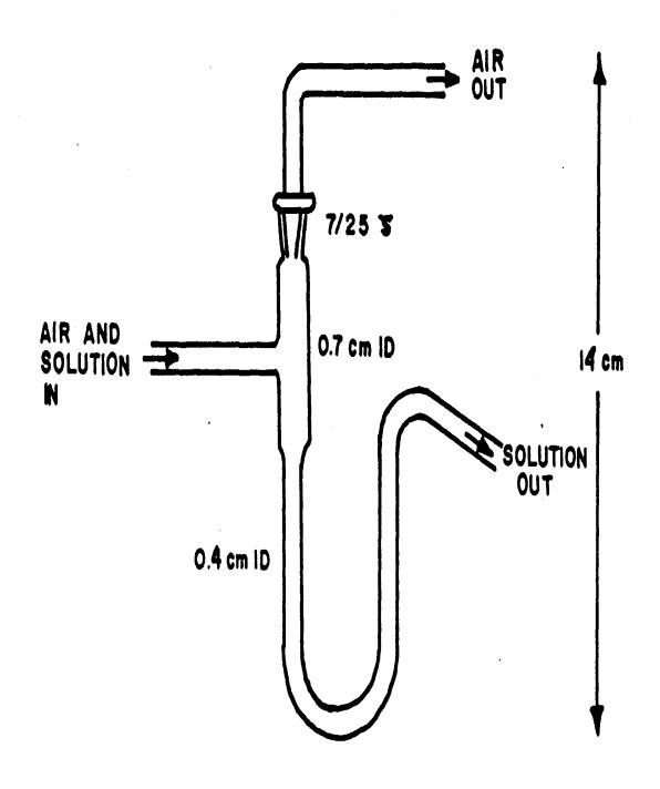
FIGURE 1. VAPOR LIQUID SEPARATOR
