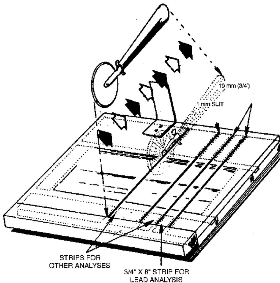
Figure 2. Diagram of filter cutting procedure.
