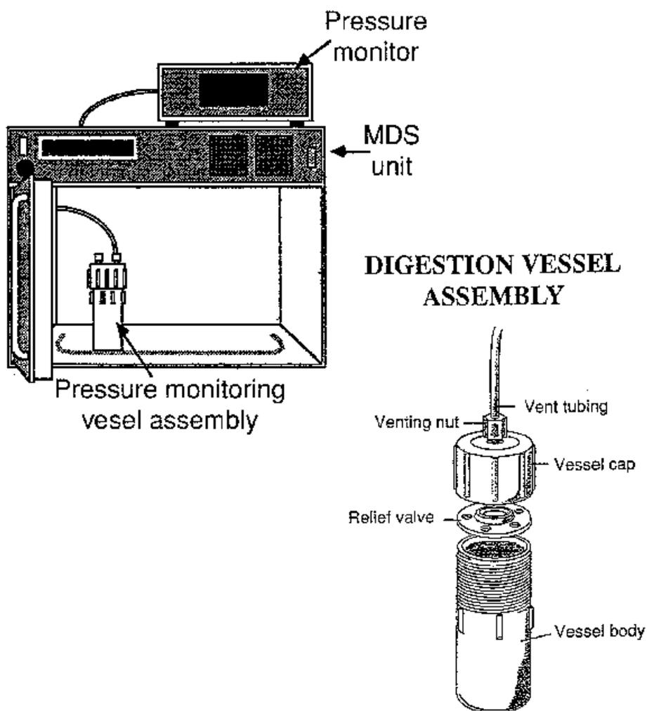
Figure 3. Example of microwave digestion system.
