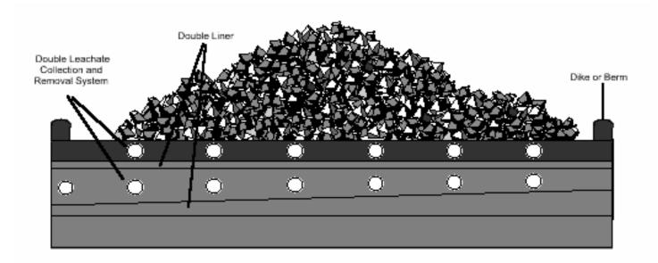
provision only requires the owner and operator of a waste pile meeting MTR to record the amount of liquids removed from the leak detection system sump at least once a week (§265.260). Note that waste piles are not subject to the emergency repair provisions for surface impoundments.
