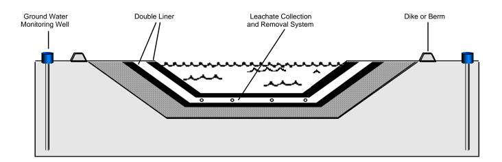
A surface impoundment must also be designed to prevent the flow of liquids over the top of an impoundment (or overtopping) and ensure the structural integrity of any dikes. Also, §264.222 requires that the owner or operator establish a site-specific leachate flow rate, called the action leakage rate (ALR), to indicate when each regulated unit's system is not functioning properly.
