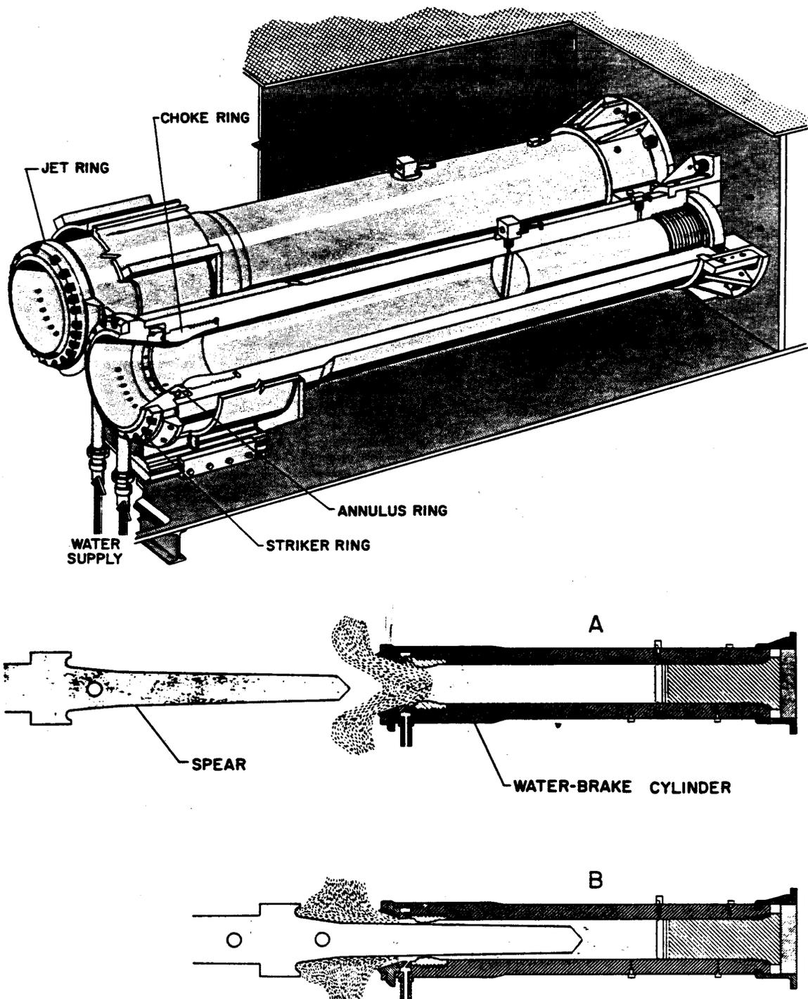
Fig. 1 Water Brakes
