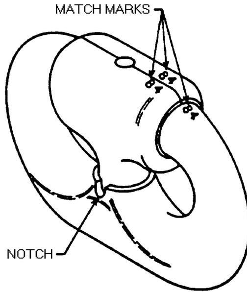
**Figure 1. Schematic Diagram of a Typical Detachable Chain Link**
