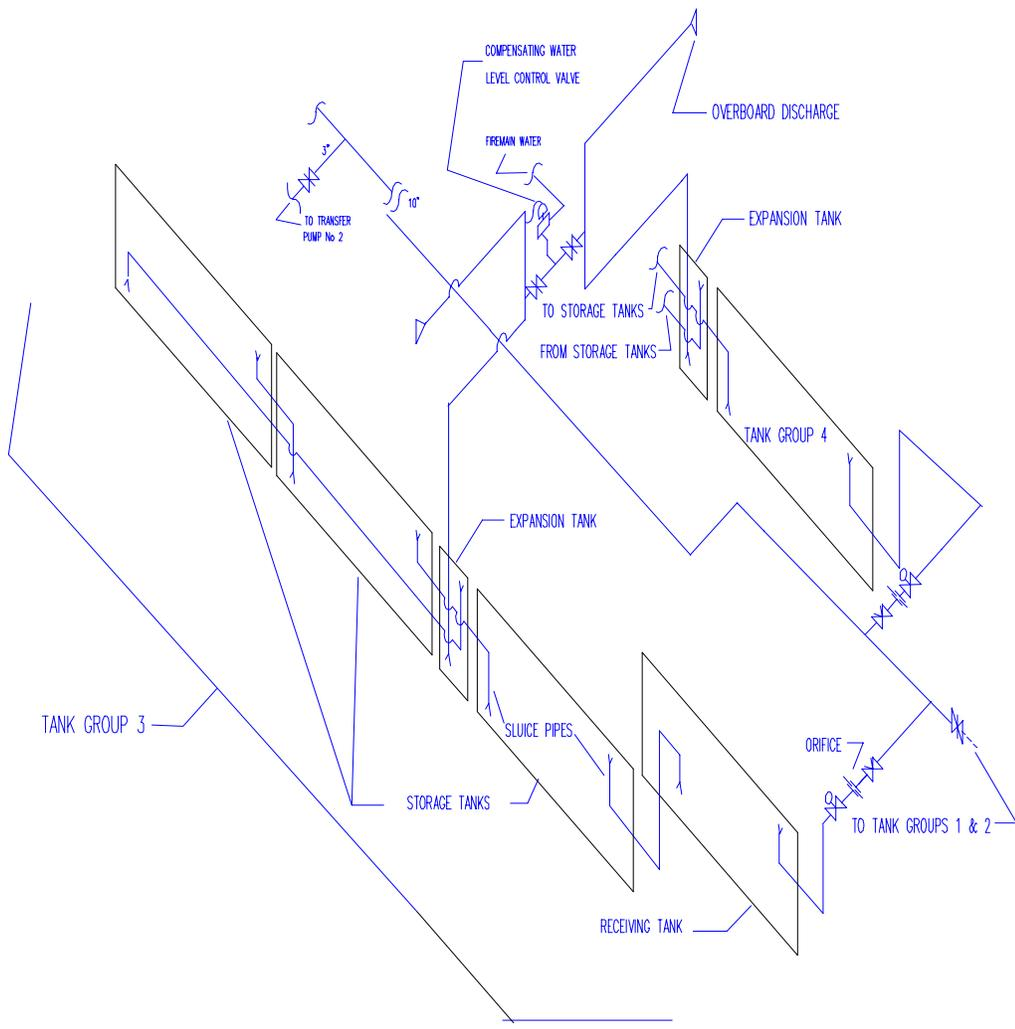
**Figure 3. Typical Port and Starboard Tank Groups with Cross-connected Overflow**
