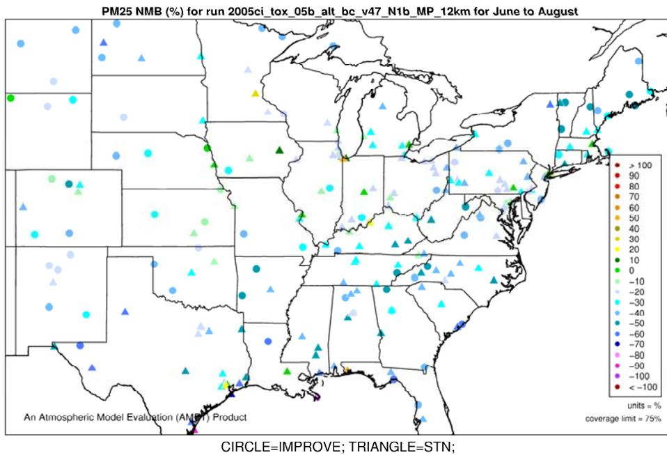
**Figure E-5. Normalized Mean Bias (%) of PM<sub>2.5</sub> by monitor for 12-km Eastern U.S. domain, Summer 2005.**
