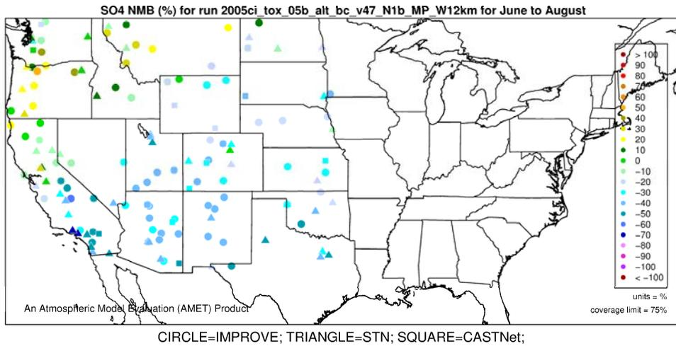
**Figure F-13. Normalized Mean Bias (%) of sulfate by monitor for 12-km Western U.S. domain, Summer 2005.**
