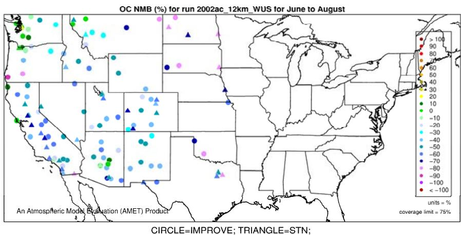
**Figure J-13. Normalized Mean Bias (%) of organic carbon by monitor for 12-km Western U.S. domain, Summer 2005.**
