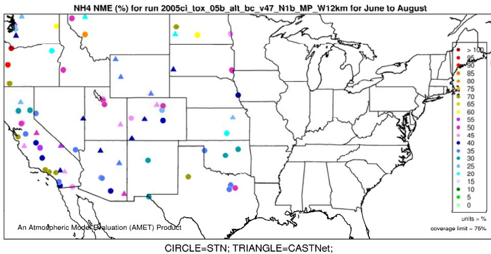
**Figure H-14. Normalized Mean Error (%) of ammonium by monitor for 12-km Western U.S. domain, Summer 2005.**
