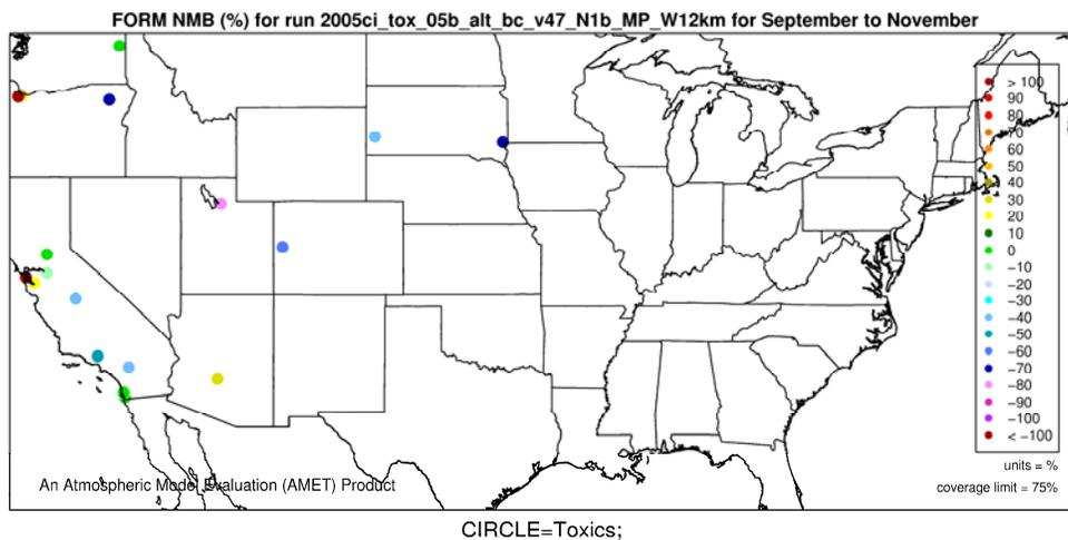
**Figure L-15. Normalized Mean Bias (%) of formaldehyde by monitor for 12-km Western U.S. domain, Fall 2005.**
