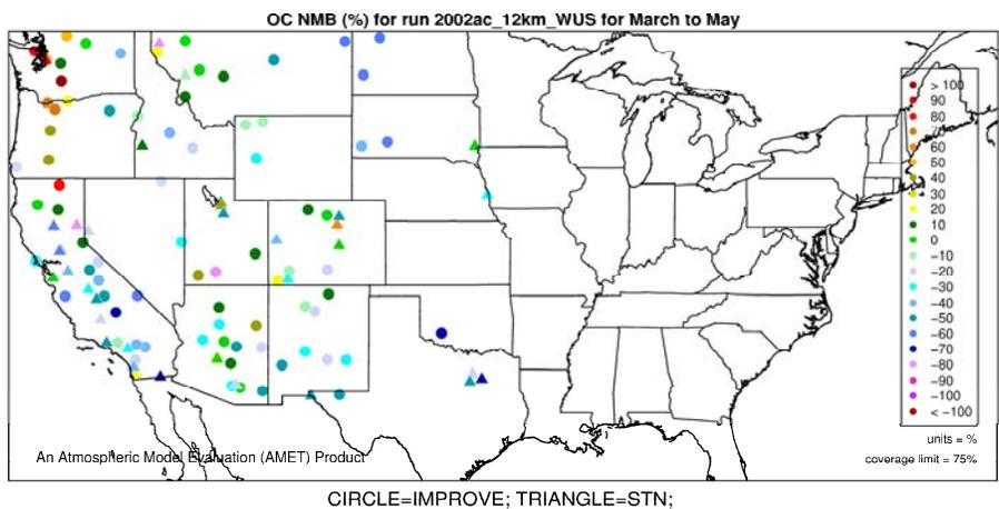
**Figure J-11. Normalized Mean Bias (%) of organic carbon by monitor for 12-km Western U.S. domain, Spring 2005.**
