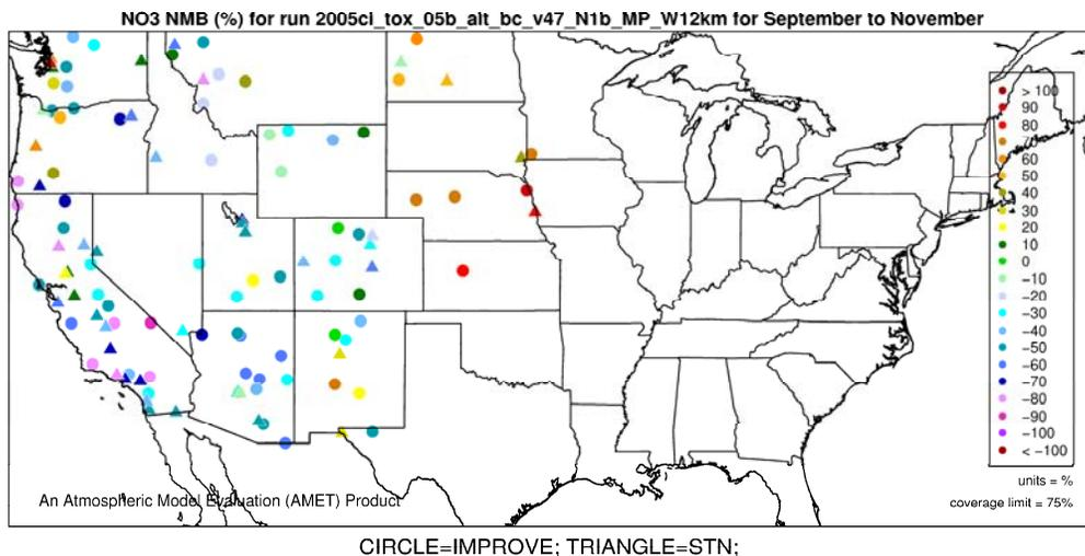
**Figure G-29. Normalized Mean Bias (%) of nitrate by monitor for 12-km Western U.S. domain, Fall 2005.**
