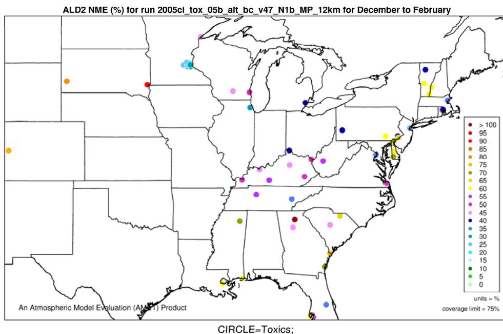
**Figure M-2. Normalized Mean Error (%) of acetaldehyde by monitor for 12-km Eastern U.S. domain, Winter 2005.**
