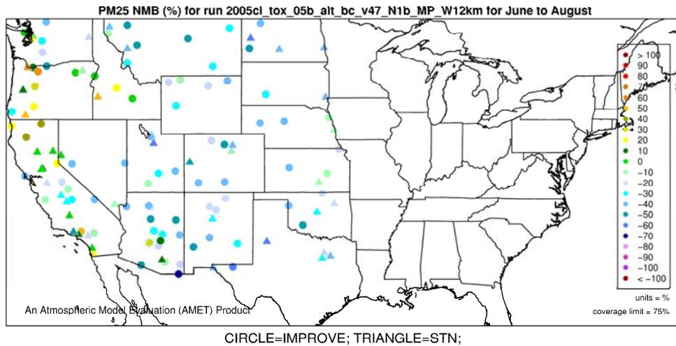
**Figure E-13. Normalized Mean Bias (%) of PM<sub>2.5</sub> by monitor for 12-km Western U.S. domain, Summer 2005.**
