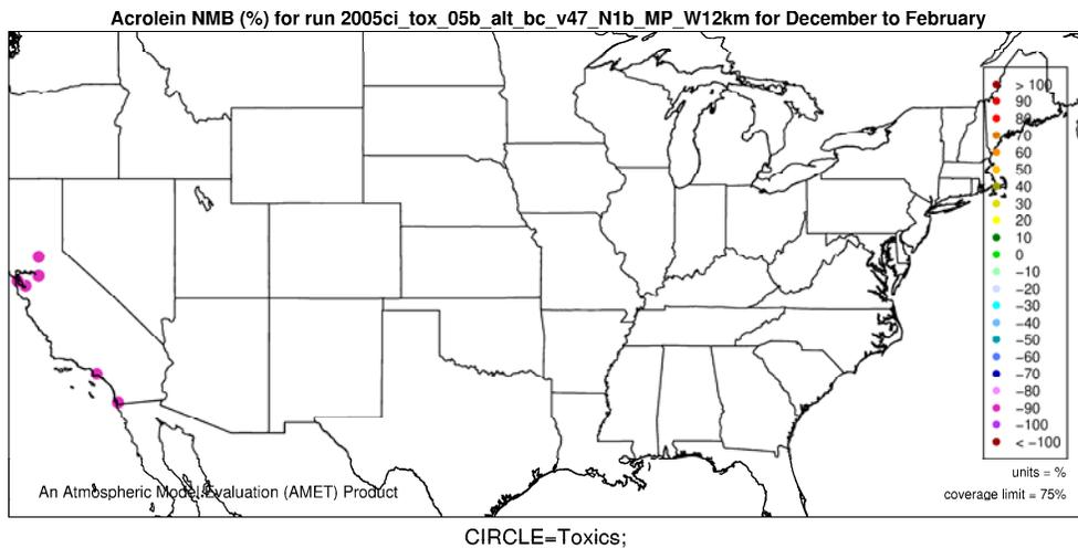
**Figure P-9. Normalized Mean Bias (%) of acrolein by monitor for 12-km Eastern U.S. domain, Winter 2005.**
