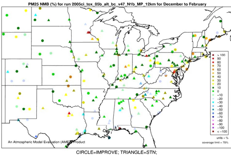
**Figure E-1. Normalized Mean Bias (%) of PM<sub>2.5</sub> by monitor for 12-km Eastern U.S. domain, Winter 2005.**
