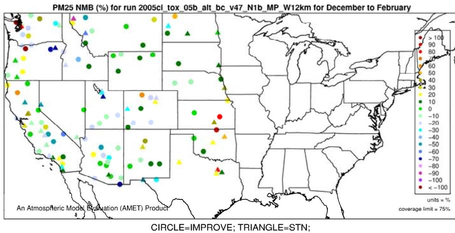
**Figure E-9. Normalized Mean Bias (%) of PM<sub>2.5</sub> by monitor for 12-km Western U.S. domain, Winter 2005.**
