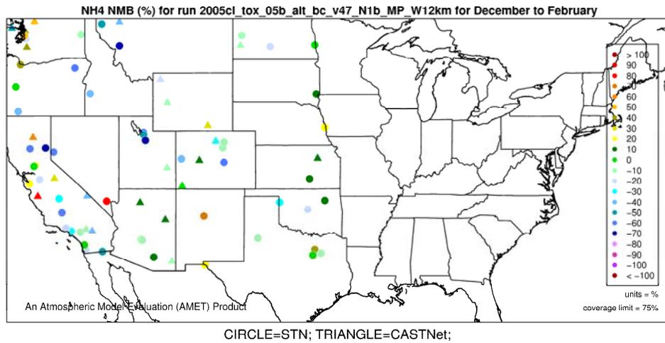
**Figure H-9. Normalized Mean Bias (%) of ammonium by monitor for 12-km Western U.S. domain, Winter 2005.**
