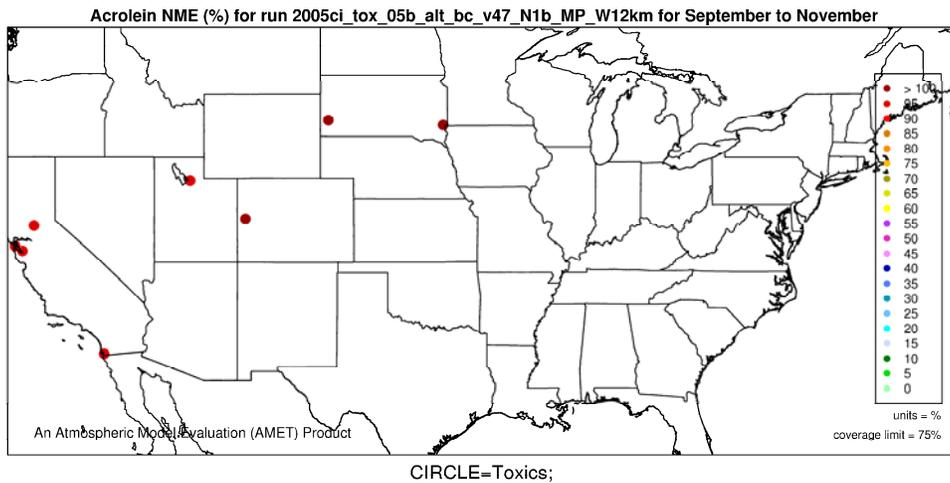
**Figure P-16. Normalized Mean Error (%) of acrolein by monitor for 12-km Western U.S. domain, Fall 2005.**
