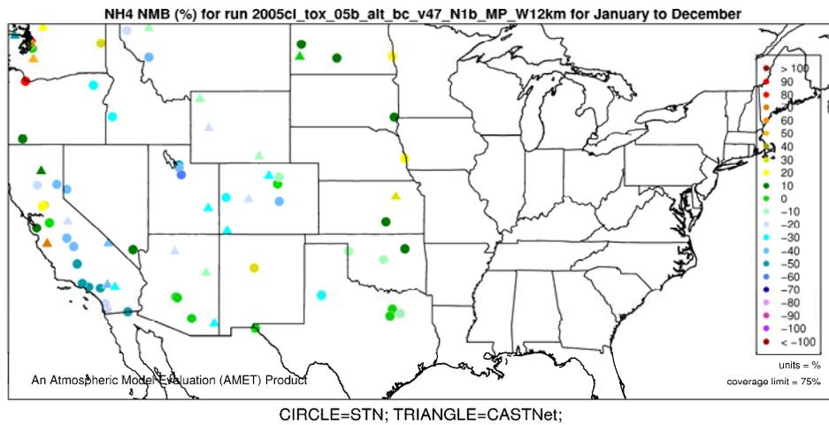
**Figure D-23. Normalized Mean Bias (%) of annual ammonium by monitor for Western U.S., 2005.**
