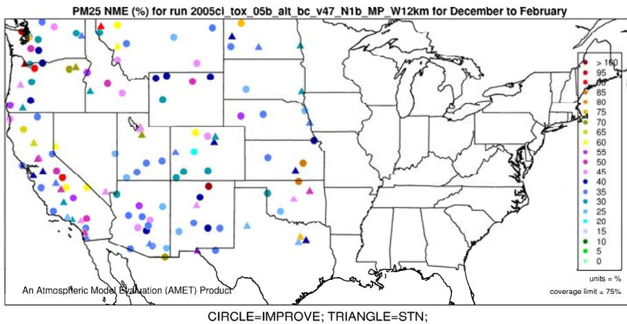
**Figure E-10. Normalized Mean Error (%) of PM<sub>2.5</sub> by monitor for 12-km Western U.S. domain, Winter 2005.**
