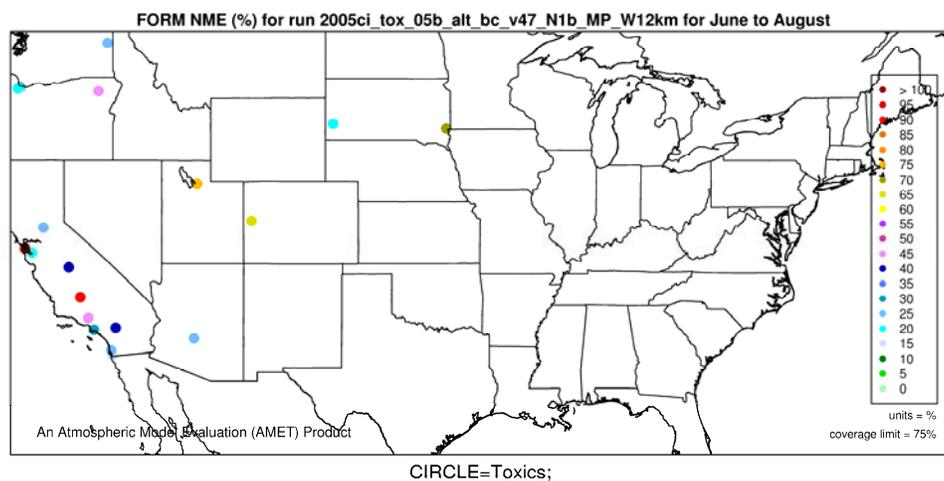
**Figure L-14. Normalized Mean Error (%) of formaldehyde by monitor for 12-km Western U.S. domain, Summer 2005.**
