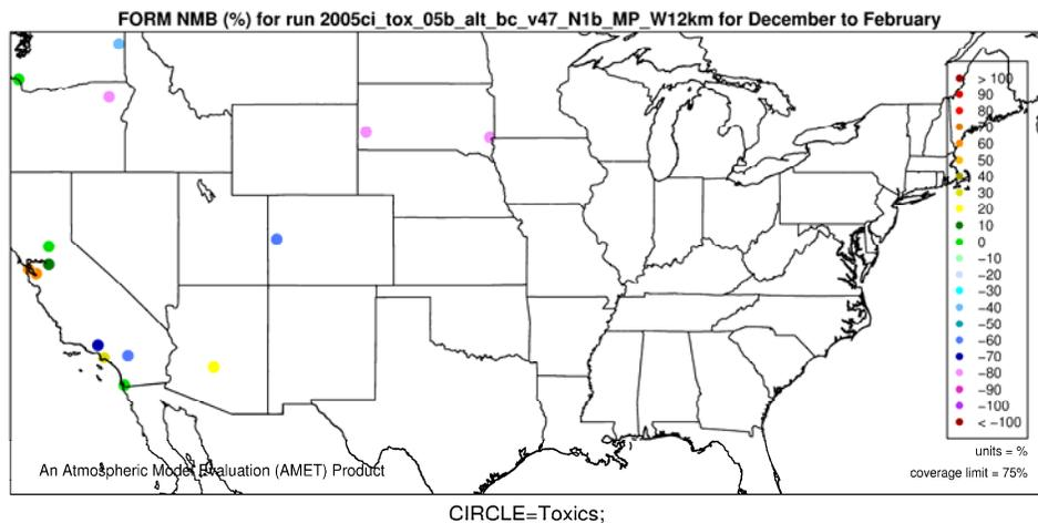
**Figure L-9. Normalized Mean Bias (%) of formaldehyde by monitor for 12-km Eastern U.S. domain, Winter 2005.**
