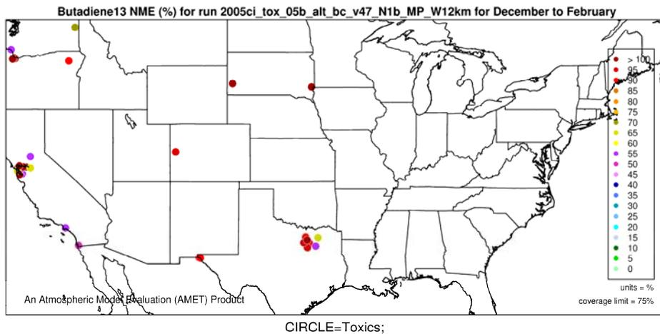
**Figure O-10. Normalized Mean Error (%) of 1,3-butadiene by monitor for 12-km Western U.S. domain, Winter 2005.**
