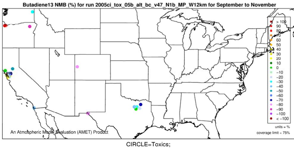
**Figure O-15. Normalized Mean Bias (%) of 1,3-butadiene by monitor for 12-km Western U.S. domain, Fall 2005.**
