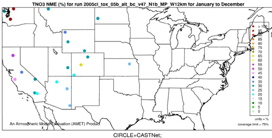
**Figure D-22. Normalized Mean Error (%) of annual total nitrate by monitor for Western U.S., 2005.**
