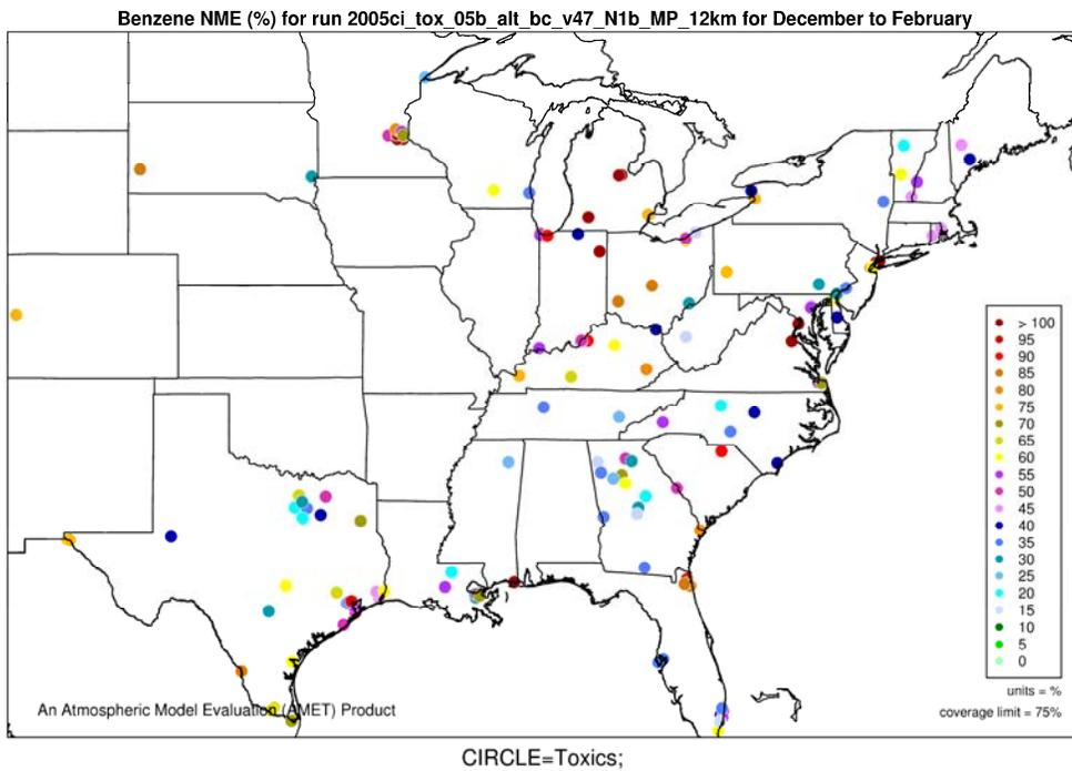
**Figure N-2. Normalized Mean Error (%) of benzene by monitor for 12-km Eastern U.S. domain, Winter 2005.**
