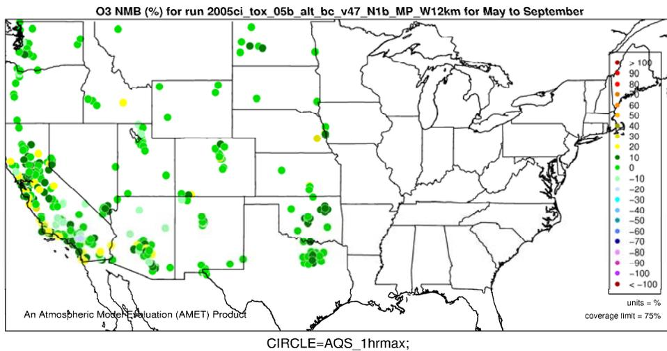
**Figure B-23. Normalized Mean Bias (%) of one-hour daily maximum ozone (40 ppb threshold) by monitor for Western U.S., seasonal aggregate 2005.**
