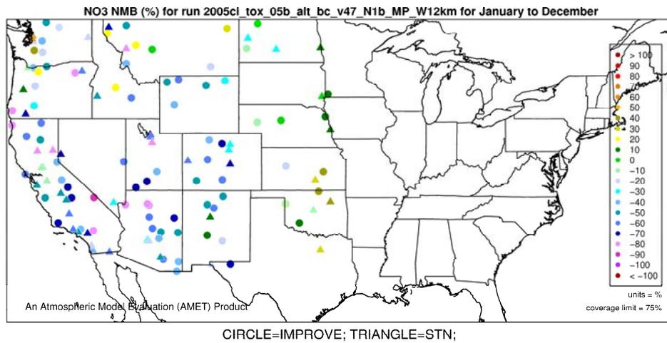
**Figure D-19. Normalized Mean Bias (%) of annual nitrate by monitor for Western U.S., 2005.**
