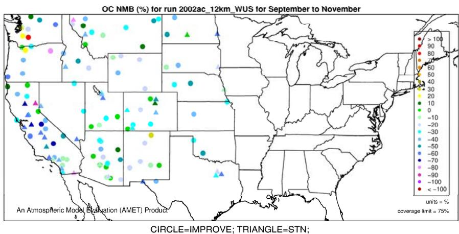
**Figure J-15. Normalized Mean Bias (%) of organic carbon by monitor for 12-km Western U.S. domain, Fall 2005.**
