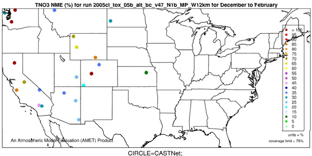
**Figure G-20. Normalized Mean Error (%) of total nitrate by monitor for 12-km Western U.S. domain, Winter 2005.**
