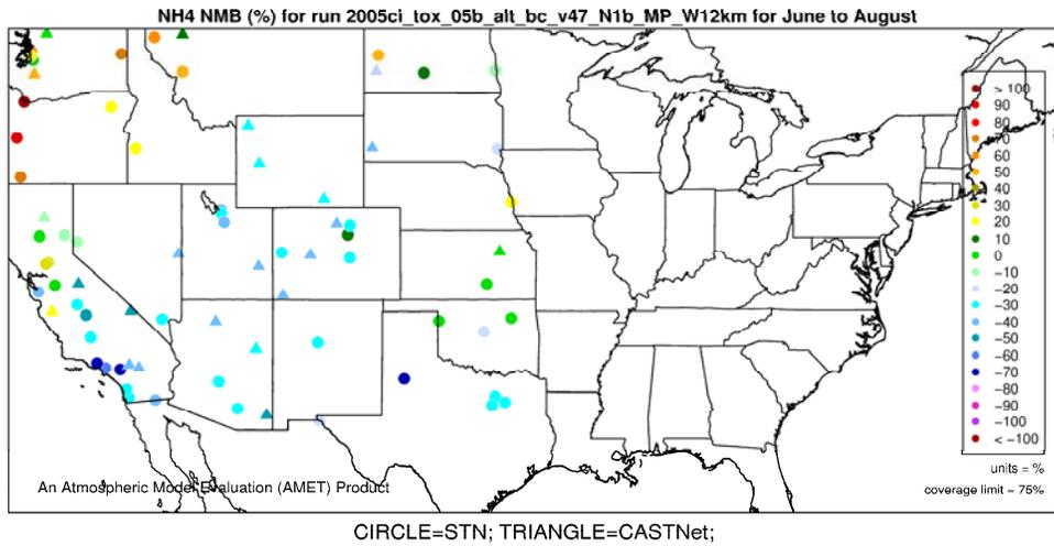
**Figure H-13. Normalized Mean Bias (%) of ammonium by monitor for 12-km Western U.S. domain, Summer 2005.**
