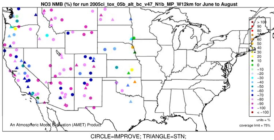
**Figure G-25. Normalized Mean Bias (%) of nitrate by monitor for 12-km Western U.S. domain, Summer 2005.**
