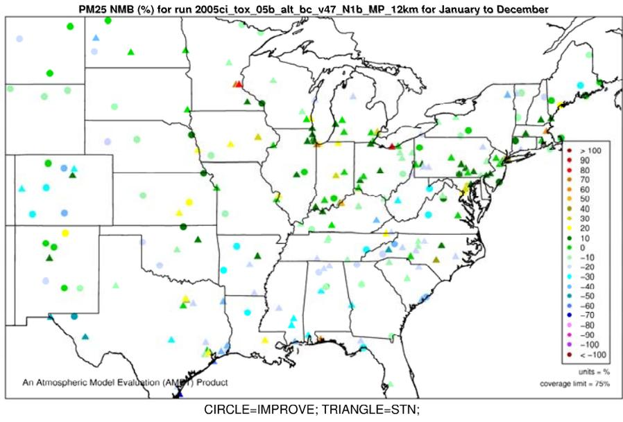
**Figure D-1. Normalized Mean Bias (%) of annual PM<sub>2.5</sub> by monitor for Eastern U.S., 2005.**
