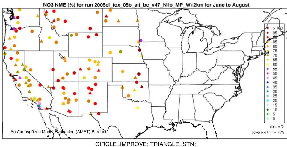
**Figure G-26. Normalized Mean Error (%) of nitrate by monitor for 12-km Western U.S. domain, Summer 2005.**
