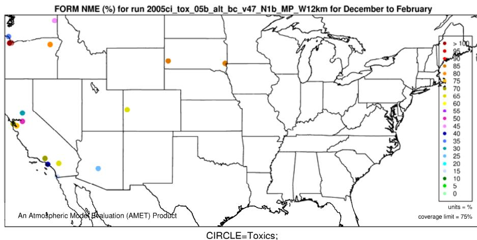
**Figure L-10. Normalized Mean Error (%) of formaldehyde by monitor for 12-km Western U.S. domain, Winter 2005.**
