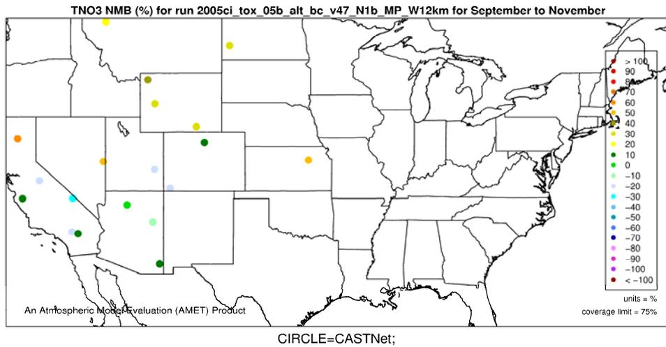
**Figure G-31. Normalized Mean Bias (%) of total nitrate by monitor for 12-km Western U.S. domain, Fall 2005.**
