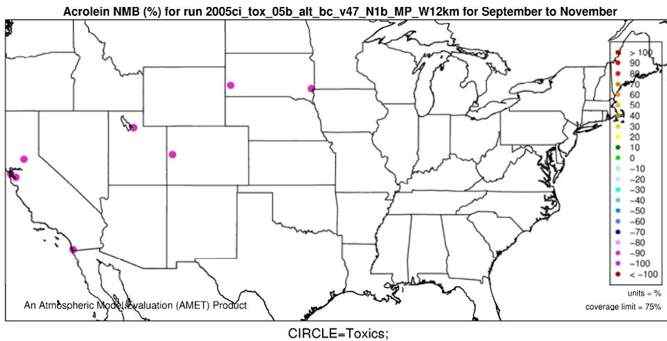
**Figure P-15. Normalized Mean Bias (%) of acrolein by monitor for 12-km Western U.S. domain, Fall 2005.**
