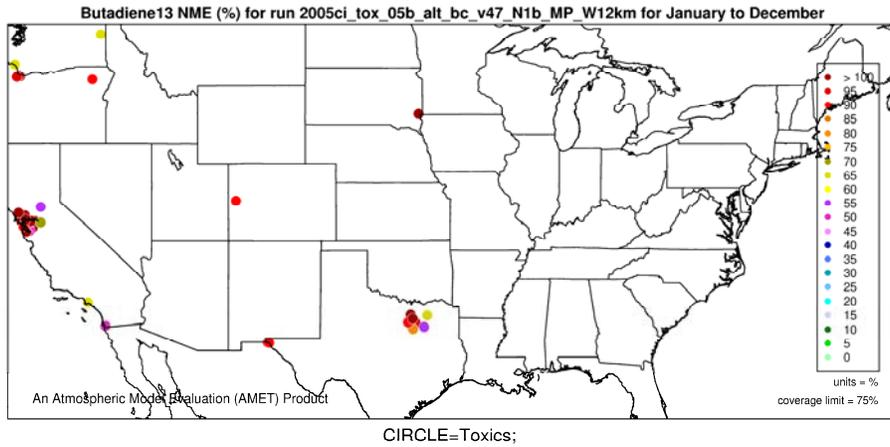
**Figure K-22. Normalized Mean Error (%) of annual 1,3-butadiene by monitor for Western U.S., 2005.**
