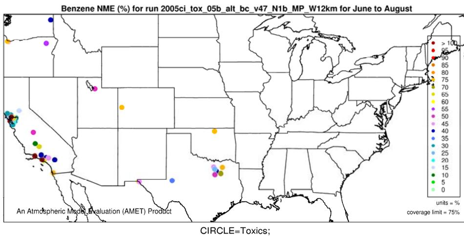
**Figure N-14. Normalized Mean Error (%) of benzene by monitor for 12-km Western U.S. domain, Summer 2005.**
