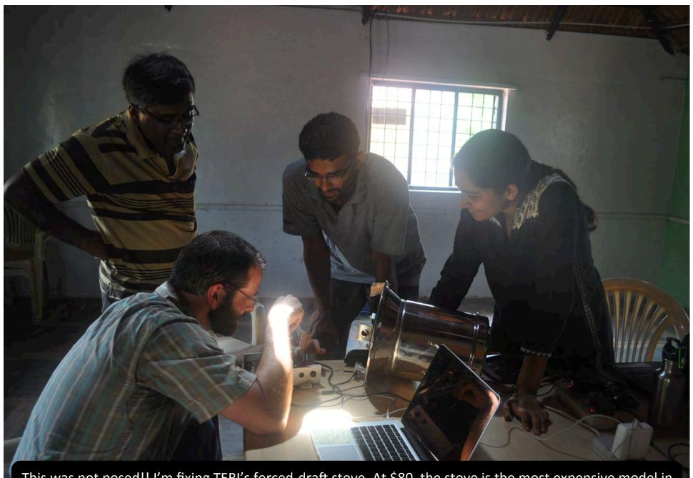
This was not posed!! I'm fixing TERI's forced-draft stove. At \$80, the stove is the most expensive model in our trial. It arrived at our test center with no fuse and 3 separate wiring faults.
