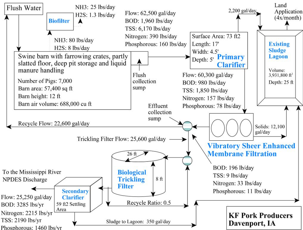
**Comparison of the Baseline Overflow to the Discharge from the Alternative Treatment System**
