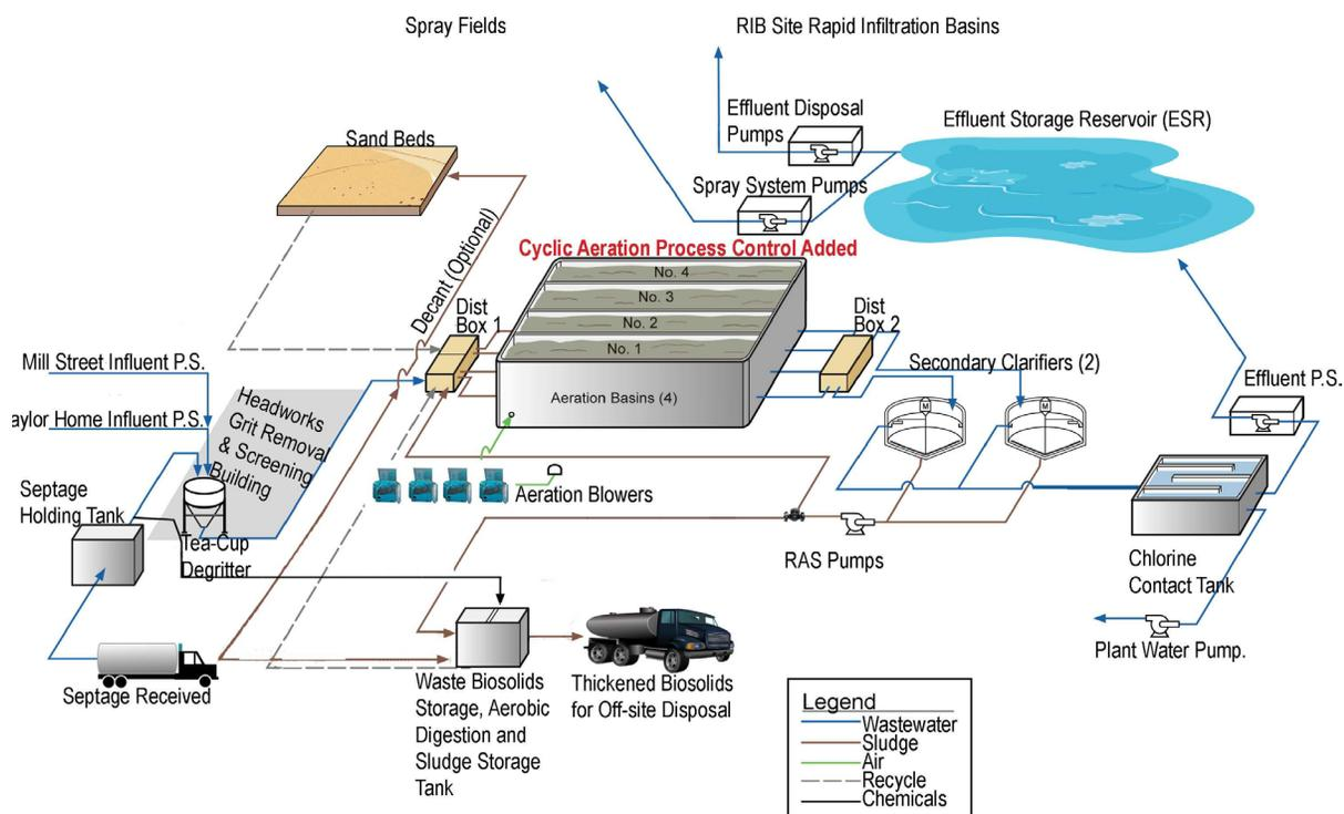
decided that it would be most cost-effective to retain the current air distribution piping and replace only the diffusers. The improvement in DO became apparent immediately upon start-up with the new diffusers, resulting in improved DO transfer and steady DO concentrations in the tanks. The improvements enabled one of the three aeration blowers to be turned off for all but the highest flow and loading conditions.
