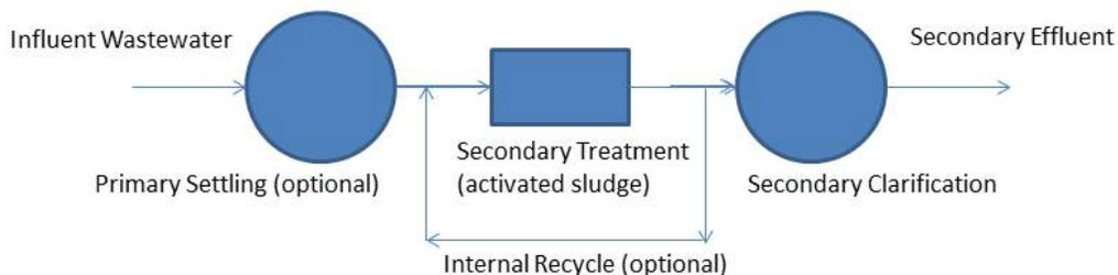
**Figure 2-4. Generalized single-reactor nitrification/denitrification liquid-phase treatment schematic**
