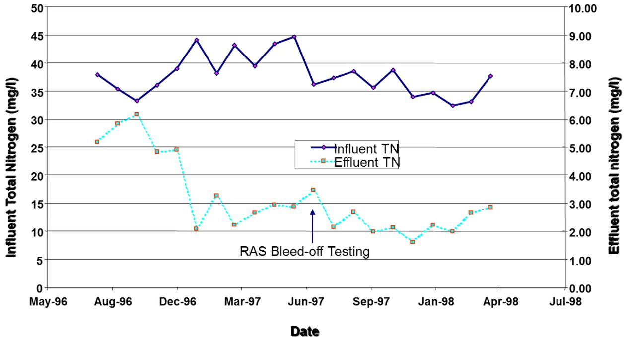
The figure below shows how the RAS bleed-off and associated increase in mixed liquor suspended solids (MLSS improved denitrification within the secondary anoxic zones. In the Blue Heron WRF, the MLSS concentration of the secondary anoxic zone was increased by about 20 percent, while the average effluent TN was reduced by nearly one-half during the test period profiled.
