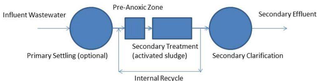
**Figure 2-2. Generalized pre-anoxic zone nitrification/denitrification liquid-phase treatment schematic**
