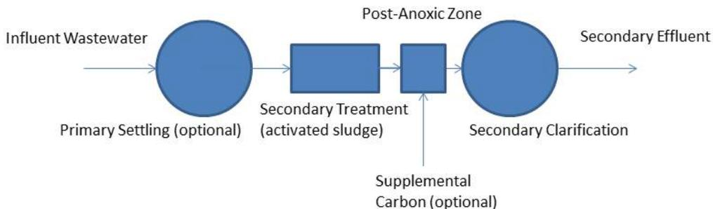
**Figure 2-3. Generalized post-anoxic zone nitrification/denitrification liquid-phase treatment schematic**
