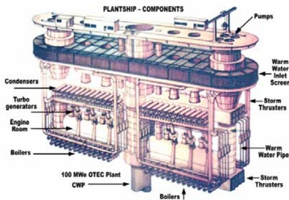
Figure 5-12. OTEC Schematic Diagram.
