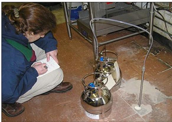
*An example of a sub-slab vapor sampling.*
