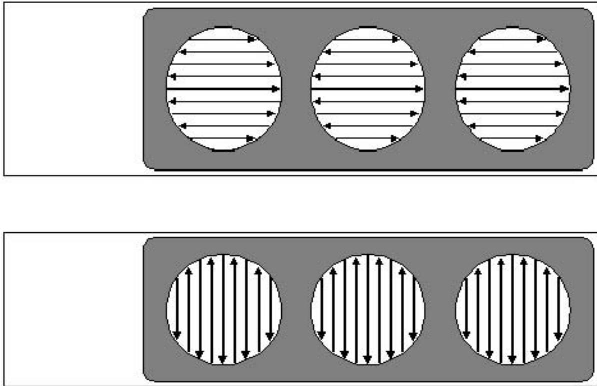
**Figure 4. Methods for Scanning a Well Slide**
