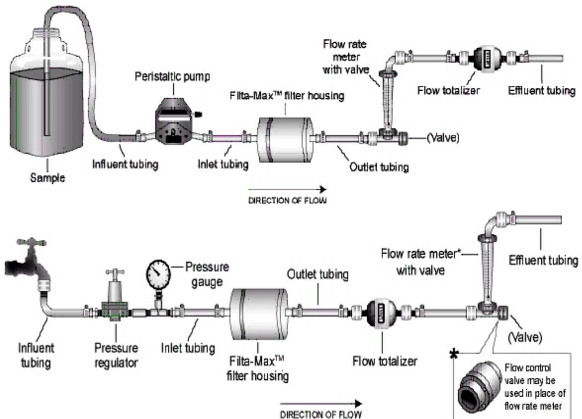
**Figure 3b. Filtration Systems for Filta-Max® filters (unpressurized source - top, pressurized source - bottom)**
