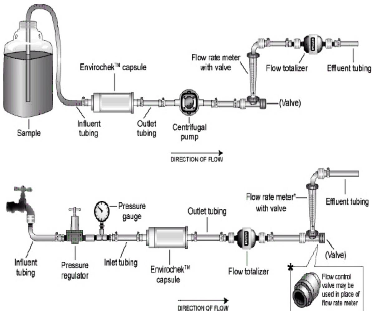
**Figure 3a. Filtration Systems for Envirochek™ or Envirochek™HV Capsule (unpressurized source - top, pressurized source - bottom)**
