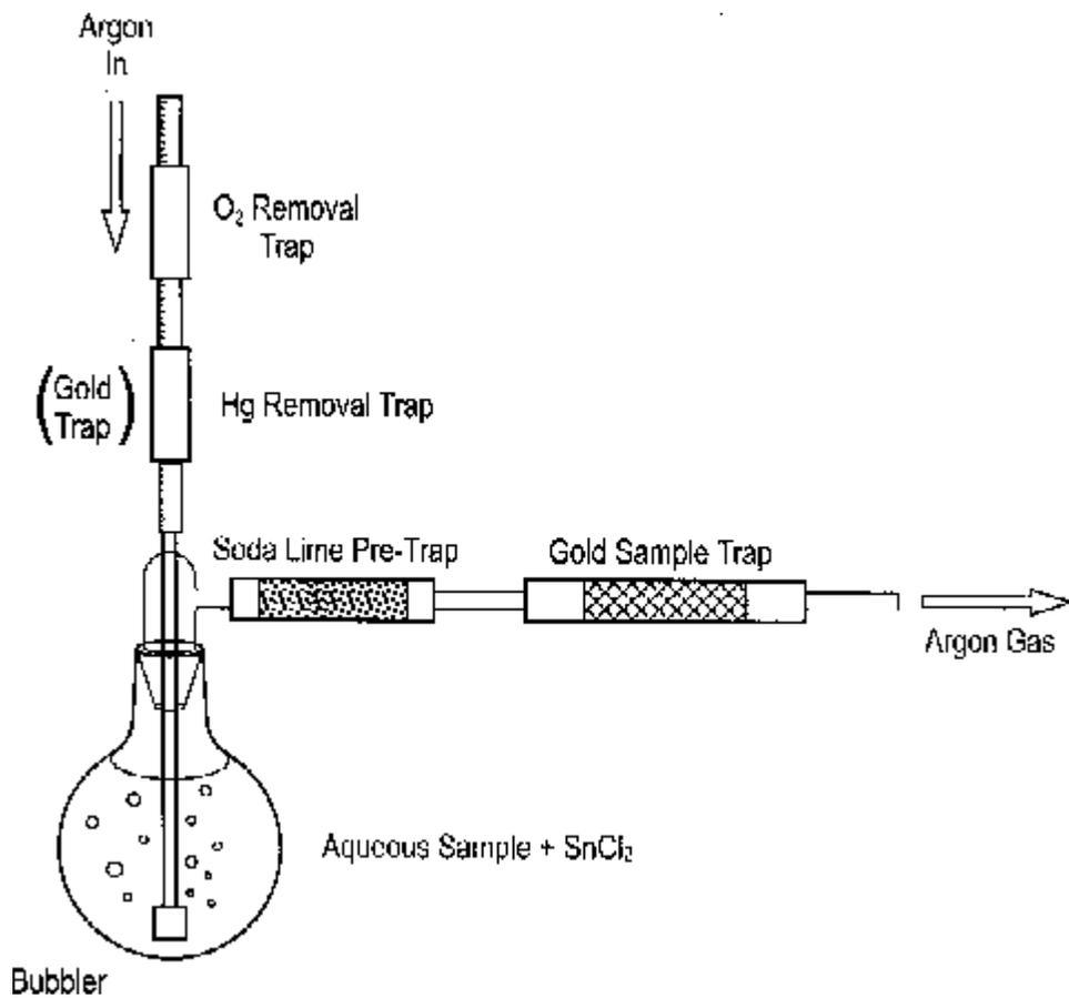
**Figure 1.** Schematic Diagram of Bubbler Setup
