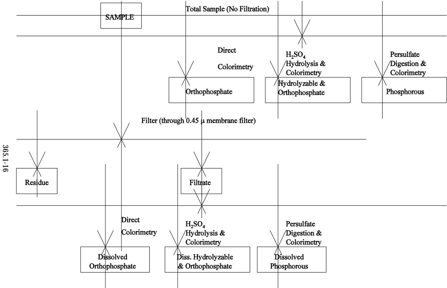
**Figure 1. Analytical Scheme for Differentiation of Phosphorous Forms**
