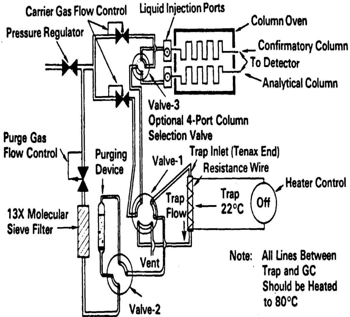
**Figure 3. Purge and trap system - purge mode.**
