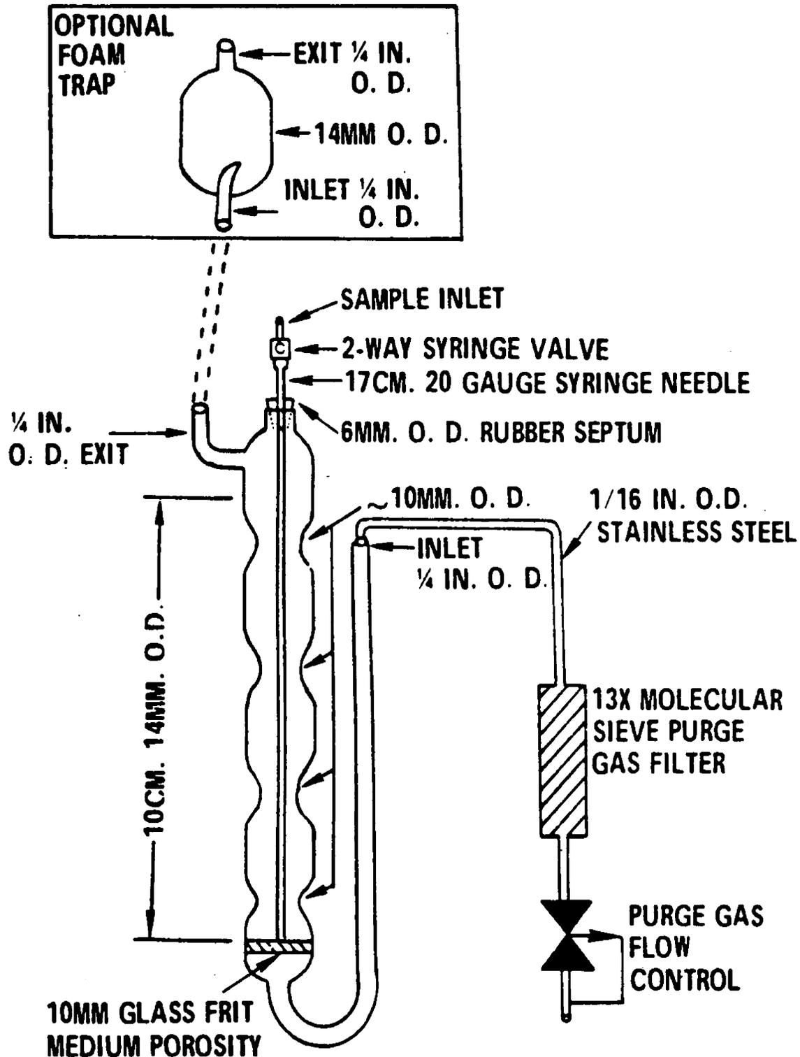
Figure 1. Purging device.
