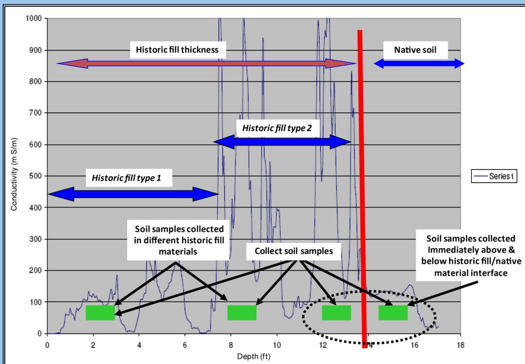
Soil Sample Intervals Selected in Field Based on Real Time Computer Readout from an EC Probe
