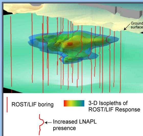
3-D Image of a Petroleum Hydrocarbon Impacted Area
