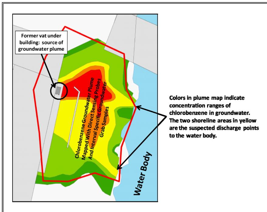
**Figure 6 – Correlation of PDB Samples and Chlorobenzene Plume Discharge Points**
