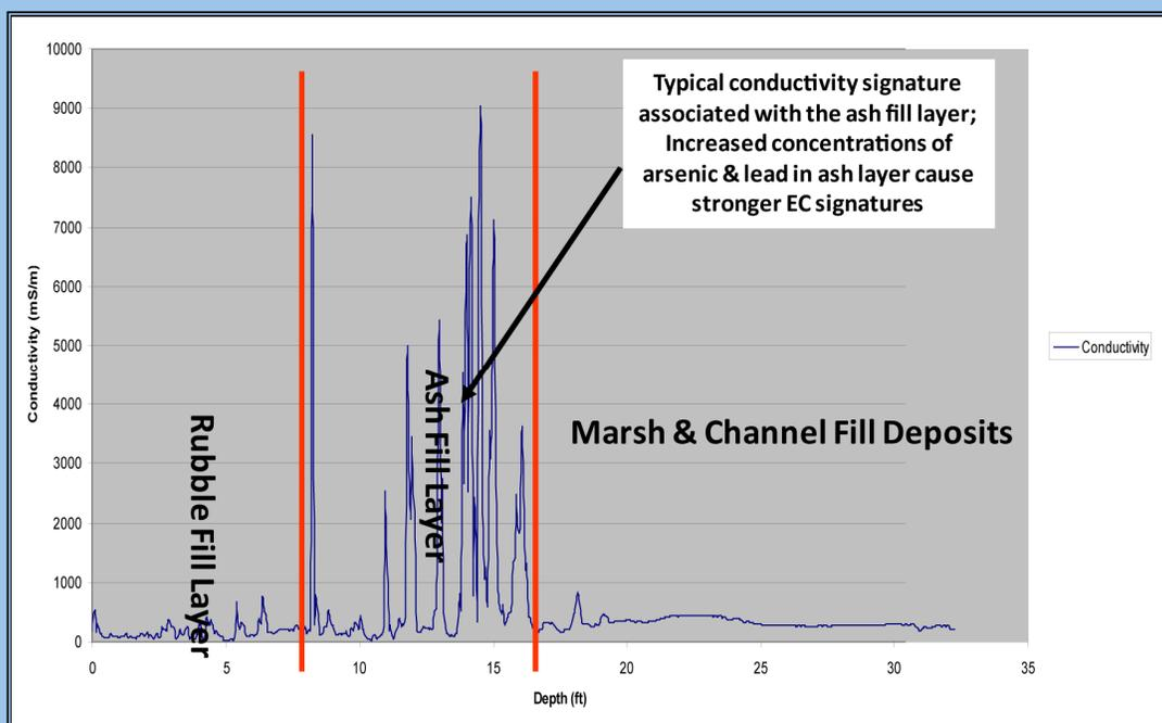
Ash Fill Layer Defined by a Clear EC Signature Caused by the Higher Conductance of the Metals in the Ash Material
