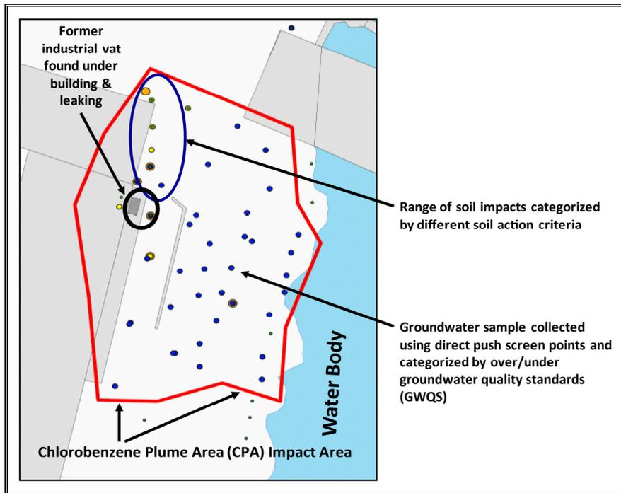
**Figure 5 – Delineated Chlorobenzene Plume**
