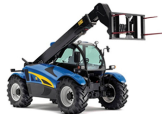
8-Ton Tele-Handler All-Terrain Forklift with DOD Compliant Spark Arrestor
