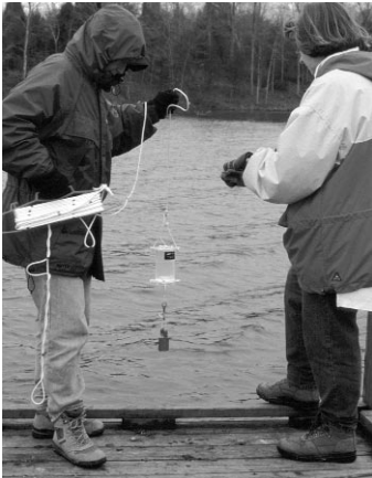
Volunteers collecting a water sample from a dock using a dissolved oxygen sampler (photo by K. Register).
