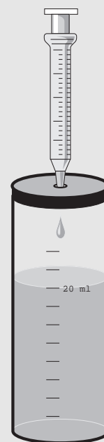
Figure 9-4. Titration of a reagent into a water sample.
