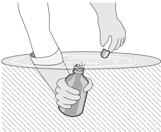
Figure 9-5. Taking a water sample for DO analysis. Point the bottle against the tide or current and fill gradually. Cap the bottle under water when full, ensuring that there are no air bubbles in the bottle (USEPA, 1997).
