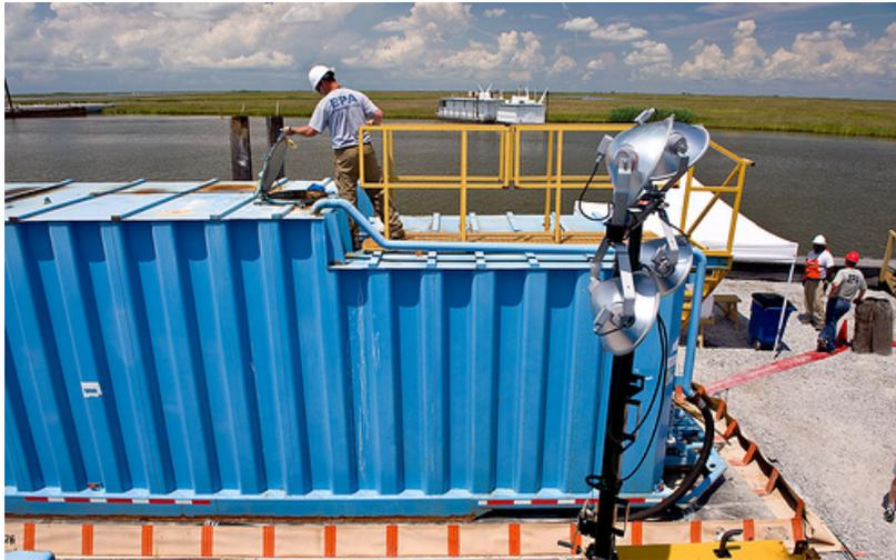
Example of a frac tank used to help oil and water separate. (EPA photo)
