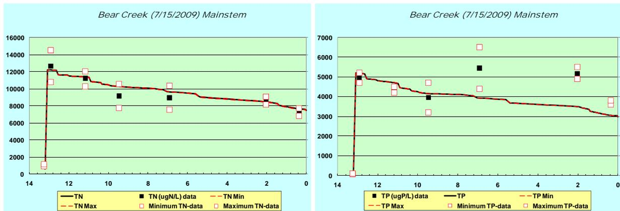
**Figure B-7. Total Nitrogen and Phosphorus Calibration in Bear Creek**
