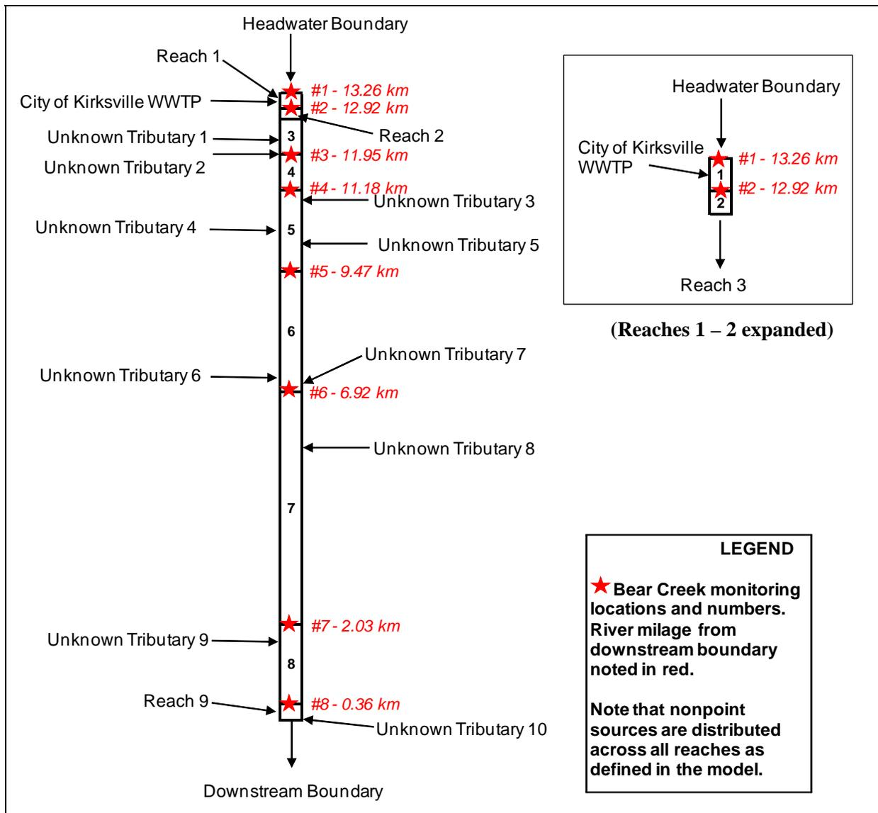
**Figure B-1. Diagram of Bear Creek QUAL2K watershed model**
