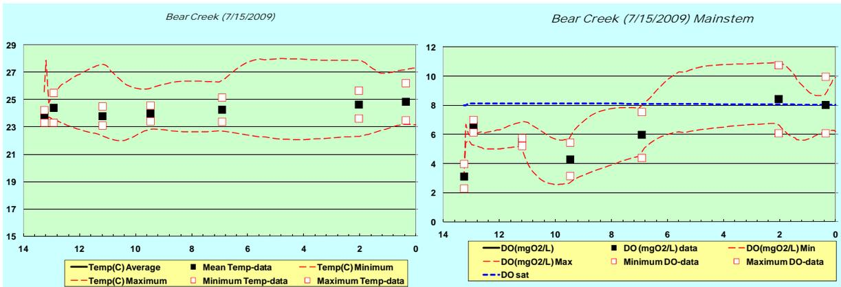
**Figure B-4. Temperature and DO Calibration in Bear Creek**
