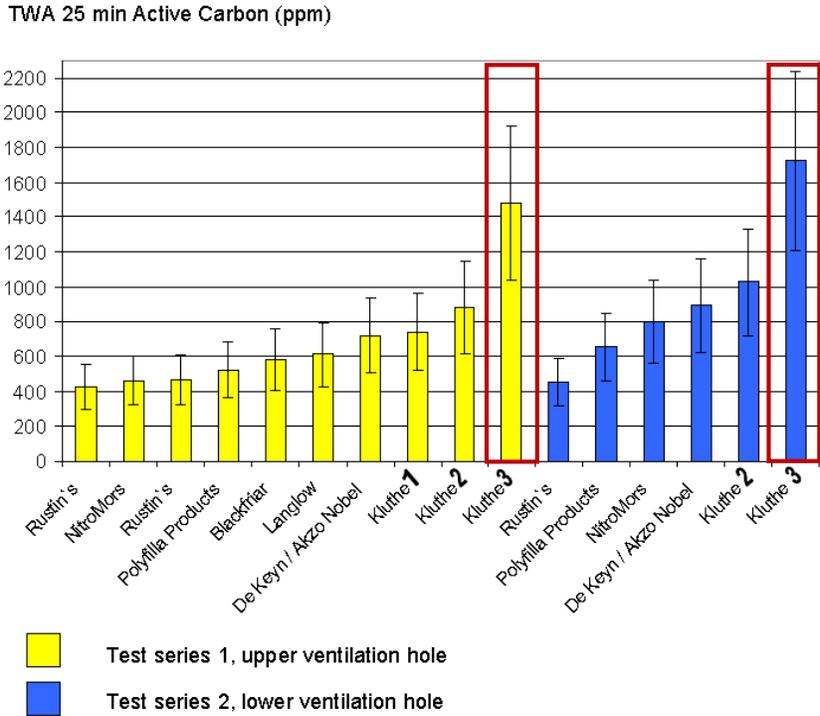
Figure 4: DCM evaporation from different paint removing products
