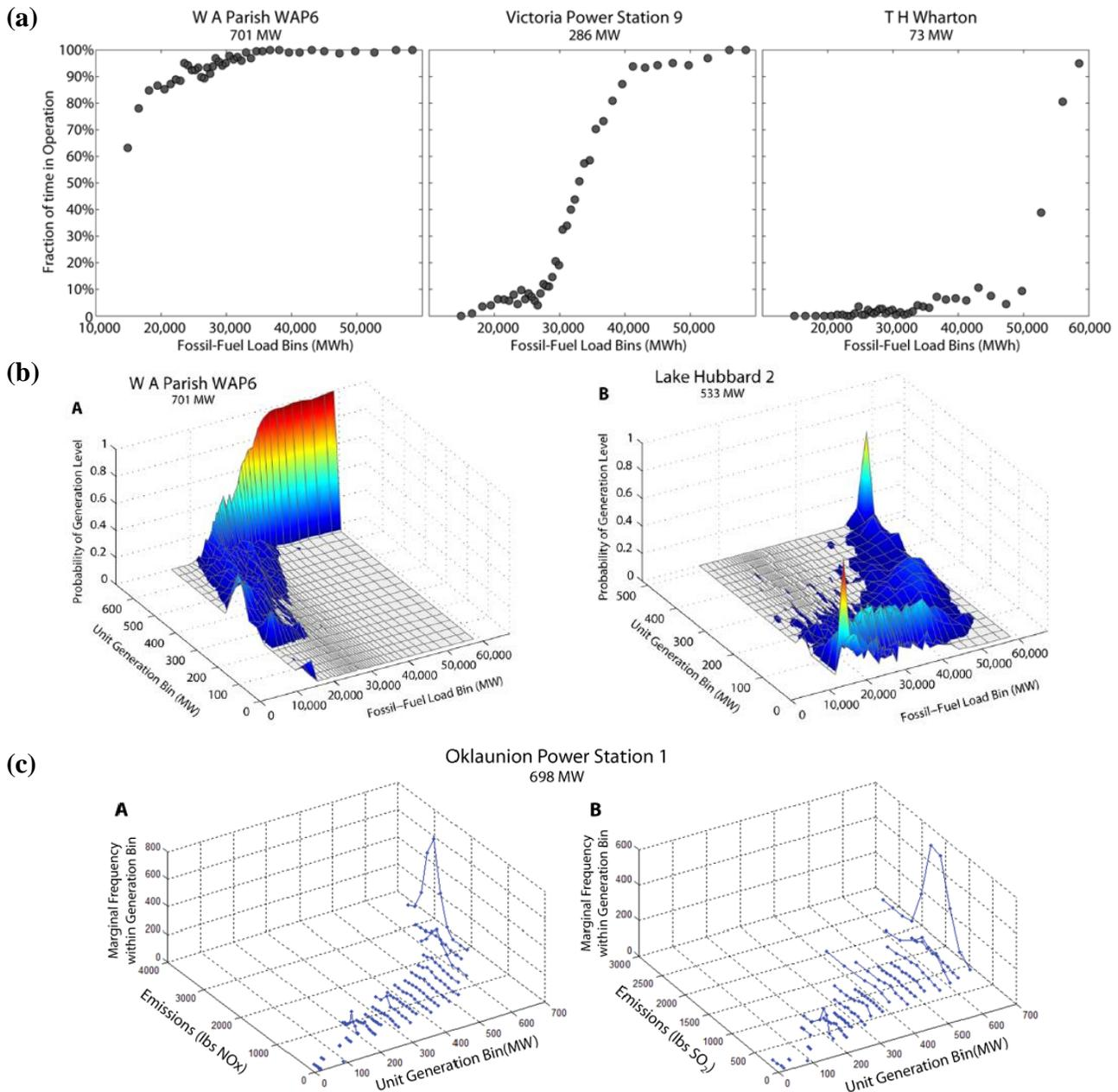
**Figure 3. AVERT's statistical algorithm: (a) determine fraction of time units are online, (b) determine generation of units at different load requirements, (c) determine emissions level at generation output**
