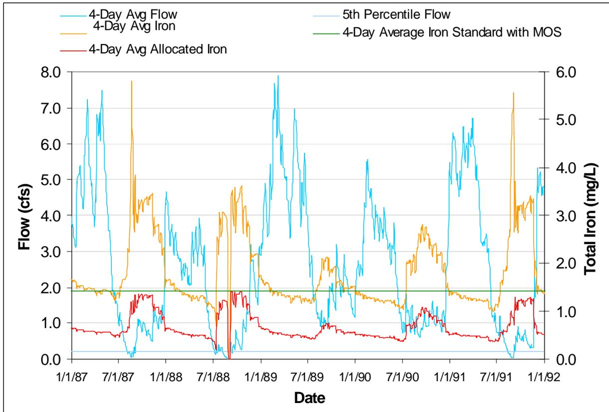
**Figure 5-2.** Baseline and TMDL conditions for iron
