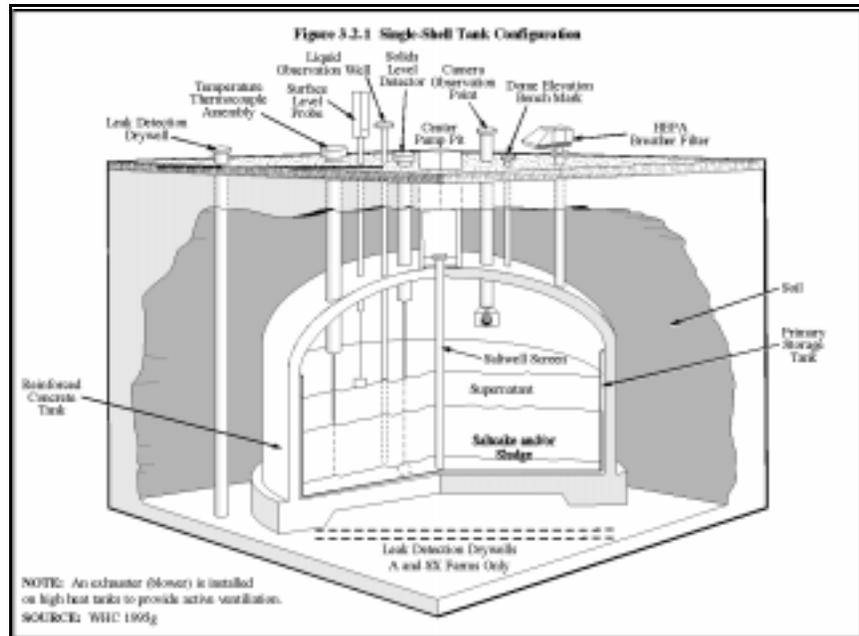
**SST Configuration Showing Various Leak Detection Devices
