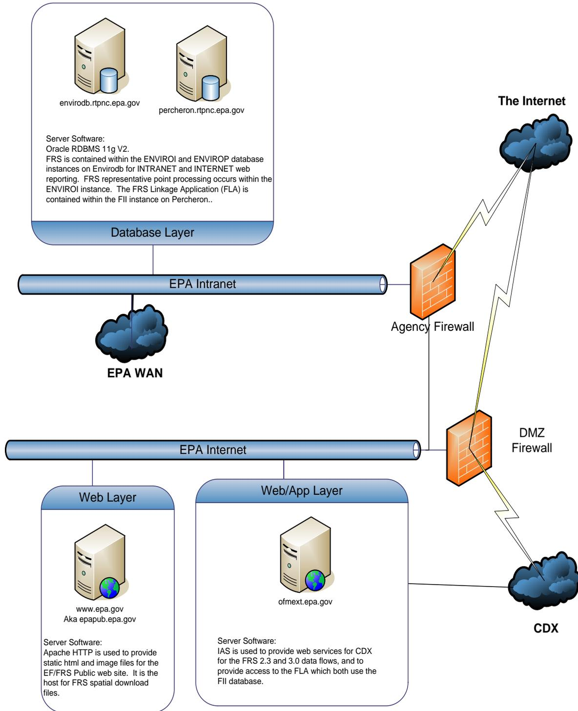
The FRS Spatial Architecture identifies the hardware and main software components that support FRS Spatial Processing.
