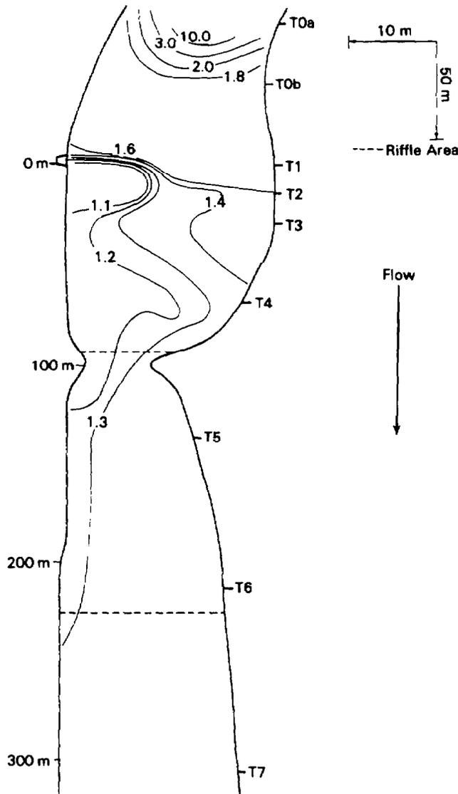
Figure 6-2. Bottom dilution contours in the Ottawa River downstream from the STP, 21 September 1982.
