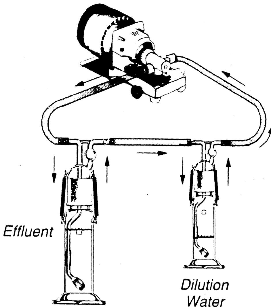
Figure 8-12. Closed loop schematic for volatile chemicals.
