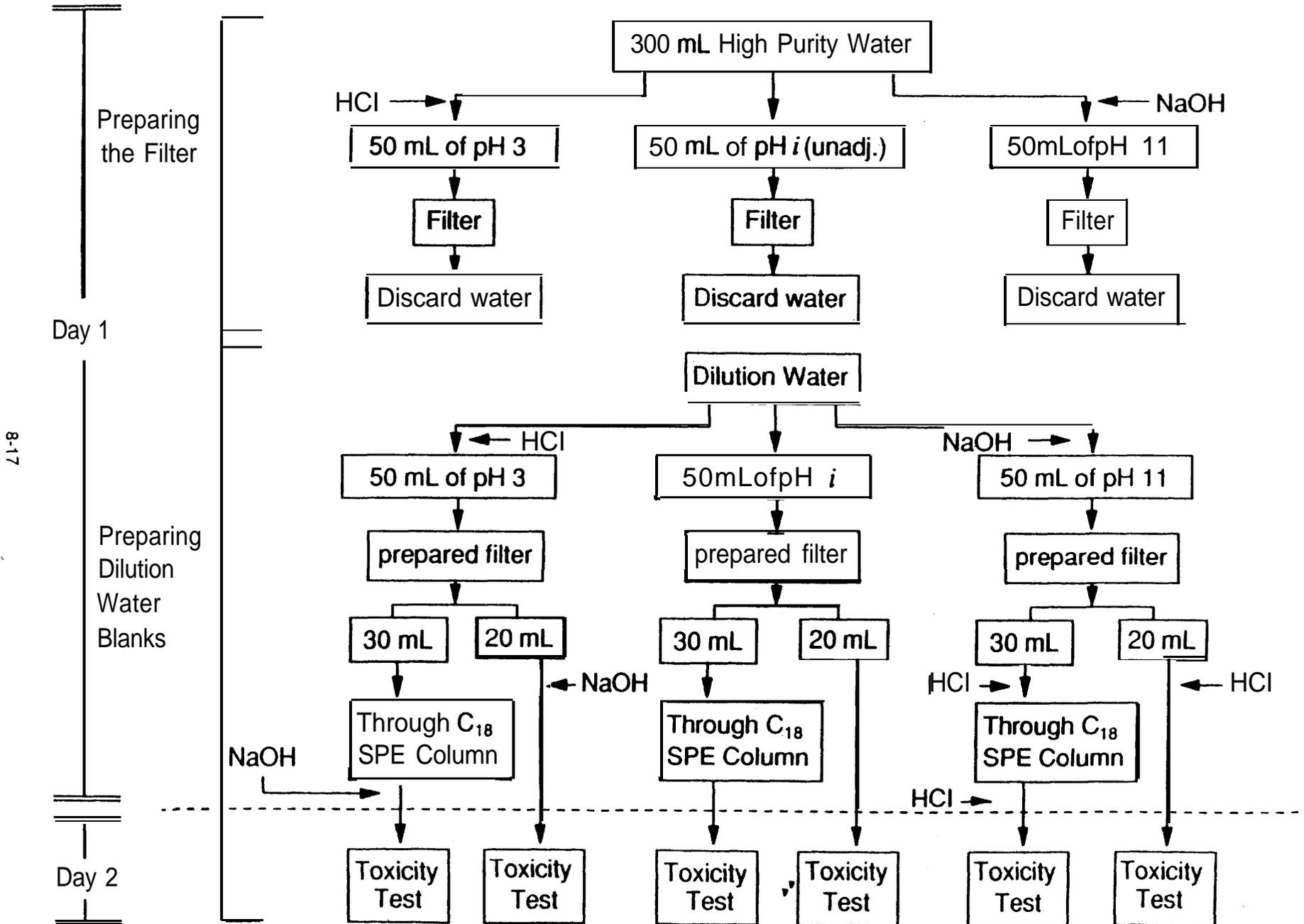
Figure 8-8. Overview of steps needed in preparing the effluent for the filtration and/or C<sub>18</sub> solid phase extraction column tests.
