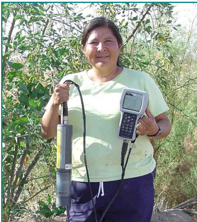
The Multi-Parameter Sonde shown in the above photograph can be used to collect pH data
