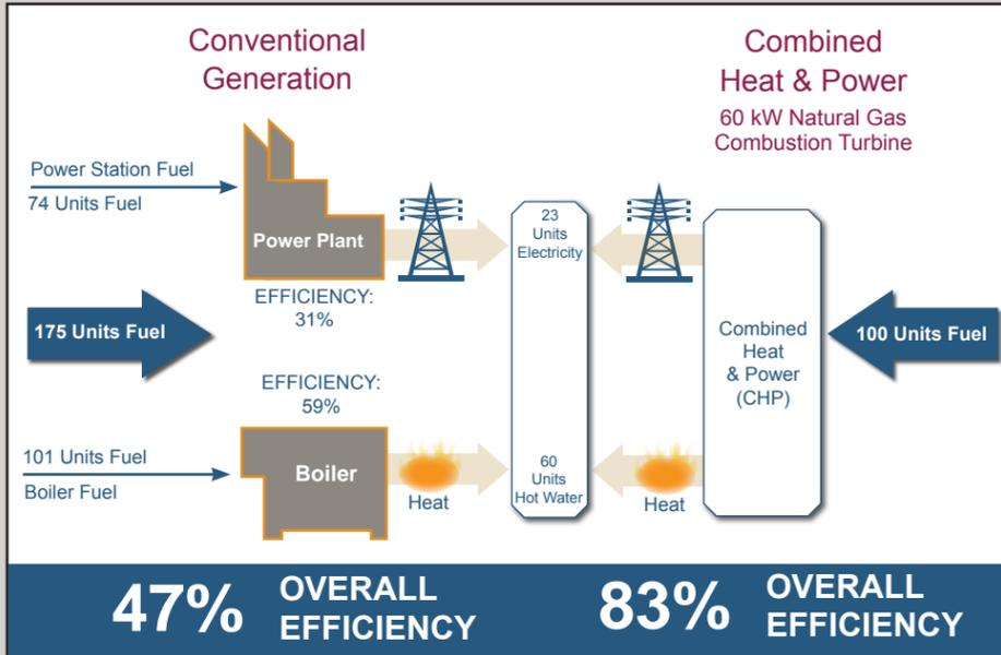
Graphical representation is only an estimate and assumes that all of the heat produced by the cogeneration unit is used by the facility, and that the unit will provide approximately 80 percent of the facility's hot water needs annually.
