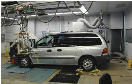
A vehicle undergoing a dynamometer test to measure vehicle emissions. (EPA photo)
