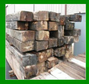
Reclaimed timber that can be milled into wood products
